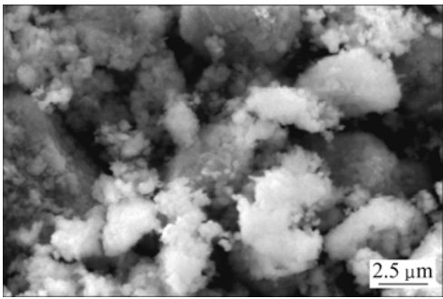
图 9 900 °C焙烧 10 h合成的 \text{Li}(\text{Ni}_{3/8}\text{Co}_{3/8}\text{Mn}_{2/8})\text{O}_2 的SEM形貌 Fig.9 SEM image of \text{Li}(\text{Ni}_{3/8}\text{Co}_{3/8}\text{Mn}_{2/8})\text{O}_2 synthesized at 900 °C for 10 h
