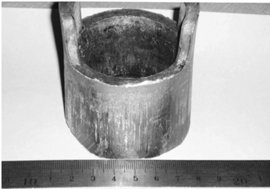
图 2 伪半固态触变模锻成形 Al/Al 2 O 3 复合材料杯形件 Fig.2 Al/Al 2 O 3 composite cup shell by thixotropic die forging in pseudo-semi-solid state
