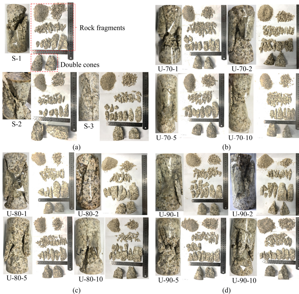
Fig. 10 Failure modes of granite specimens: (a) Monotonic loading tests; (b) \sigma_p level of 70% of UCS; (c) \sigma_p level of 80% of UCS; (d) \sigma_p level of 90% of UCS
