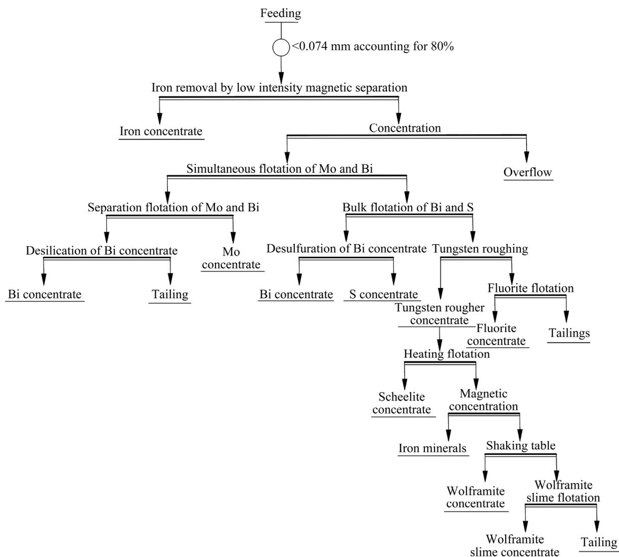
Fig. 13 Main process of Shizhuyuan Beneficiation Plant before 2015 (Drawing based on Ref. [118])
