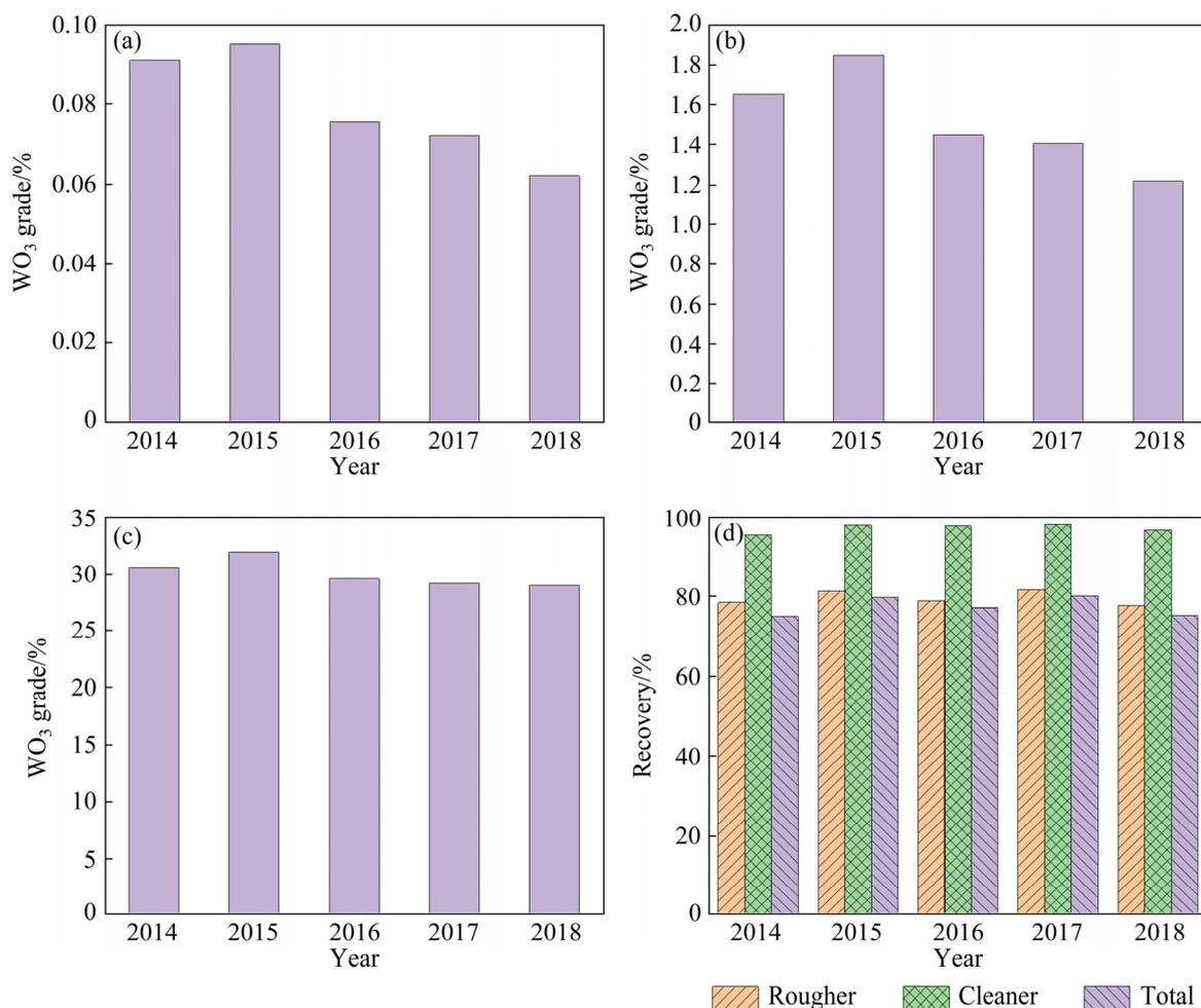
**Fig. 16** Technical indicators of tungsten beneficiation: WO<sub>3</sub> grades of feeding (a), rougher concentrate (b) and concentrate (c), and recovery of rougher, cleaner and total (d) [127]
