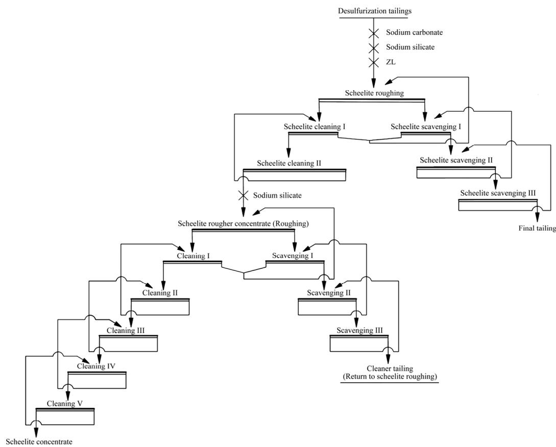
Fig. 15 Scheelite flotation process of Xianglushan Beneficiation Plant (Drawing based on Ref. [123])
