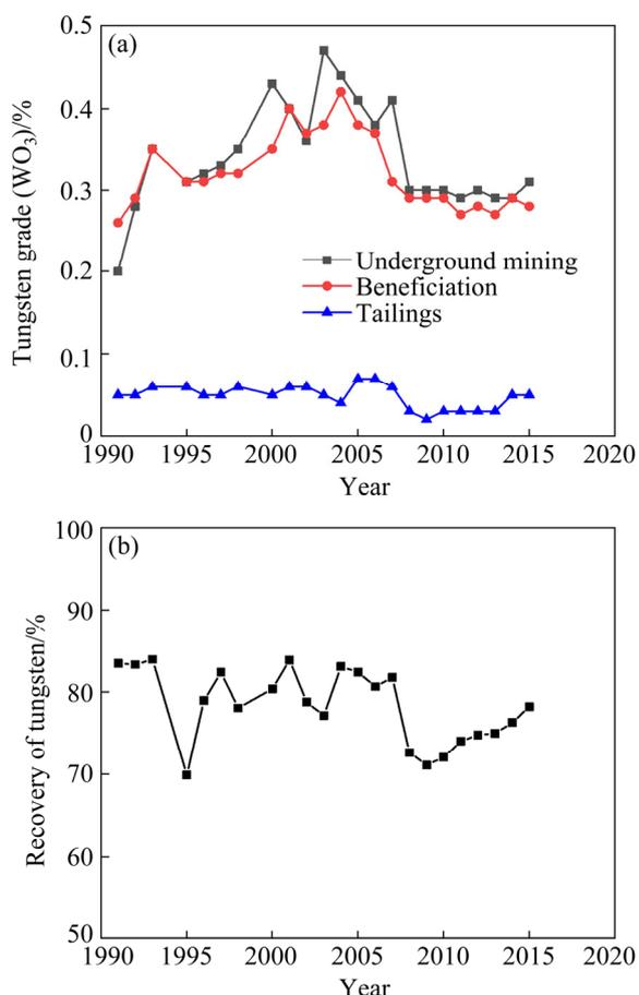
**Fig. 3** Fluctuations in tungsten grade (a) and recovery of tungsten from beneficiation (b) [39]
