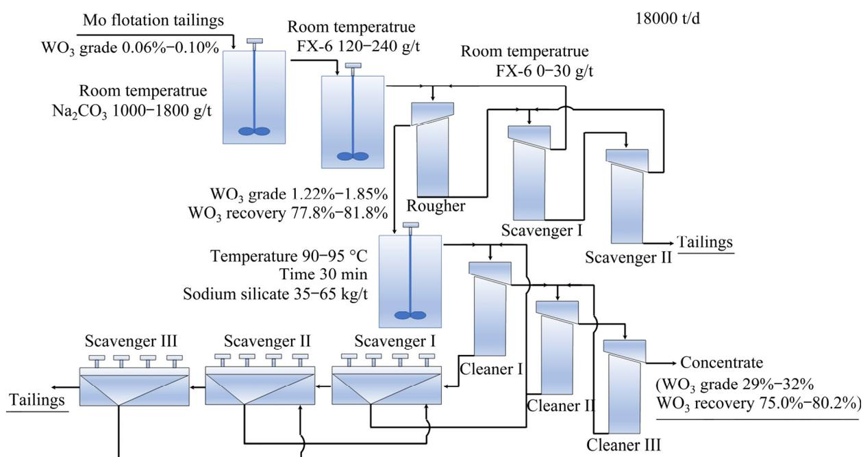
**Fig. 17** Flowsheet of recovery of tungsten from molybdenum tailings (Drawing based on Ref. [127])
