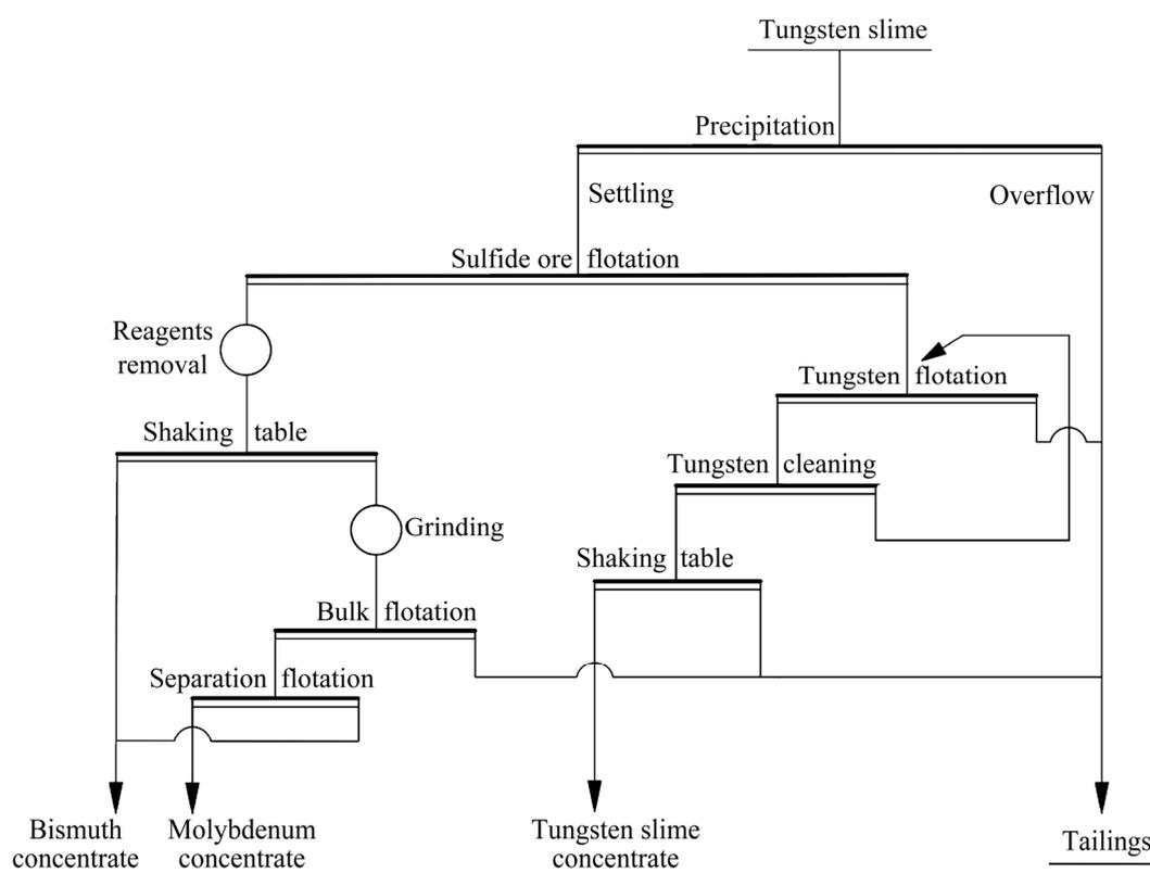
Fig. 12 Recovery process of tungsten slime (Drawing based on Ref. [120])
