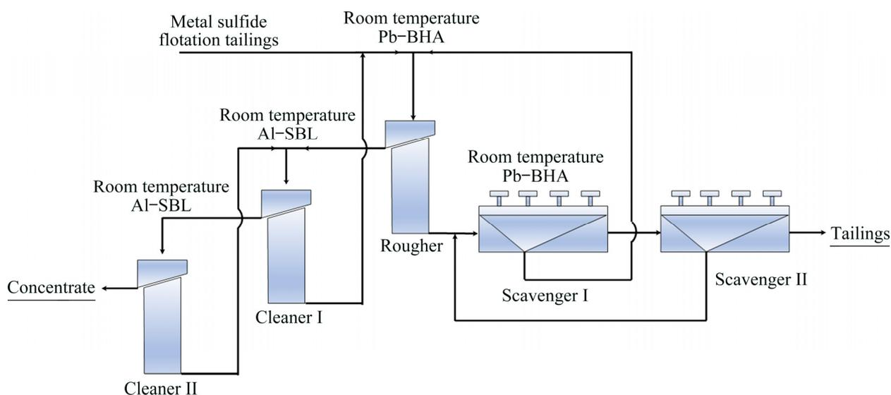
**Fig. 14** Flowsheet of recovery of tungsten from molybdenum tailings [88,122]
