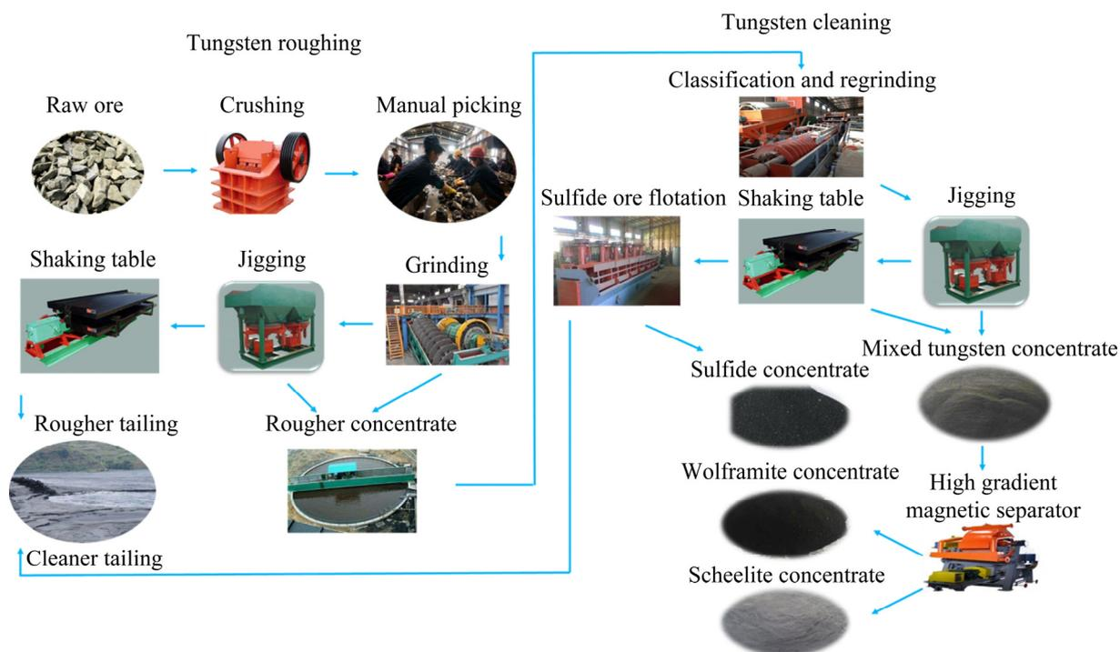
**Fig. 11** Main process of Dajishan Beneficiation Plant (Drawing based on Ref. [119])
