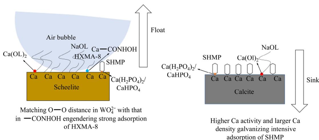
**Fig. 8** Schematic diagram of separation mechanism in novel reagent scheme (Reprinted with permission from Ref. [80])
