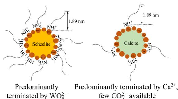
**Fig. 9** Schematic diagram of adsorption behavior of DDA species on scheelite and calcite mineral surfaces (Reprinted with permission from Ref. [83])
