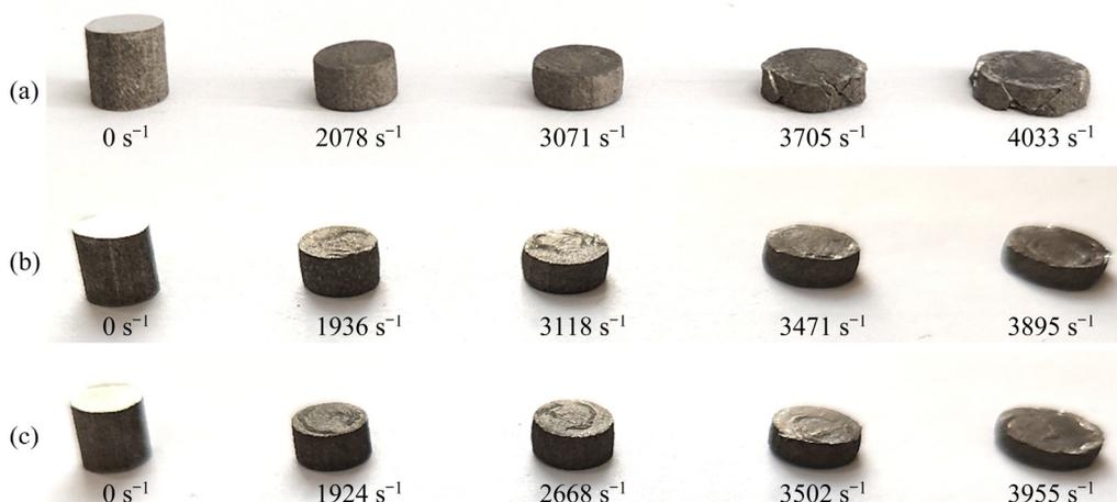
**Fig. 6** Photographs of solution-treated Mg- $x$ Gd-3Y-0.5Zr samples after dynamic compression under different strain rates: (a)  $x=6.5$ ; (b)  $x=7.5$ ; (c)  $x=8.5$
