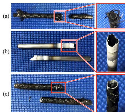
**Fig. 1** Nb lined SiC/SiC composite tubes after tensile testing at room temperature (a) and 1200 °C (c), and Nb tube after tensile testing at 1200 °C (b)
