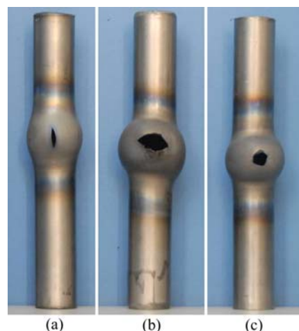
Fig. 10 Three typical forms of fracture: (a) Axial fracture; (b) Hoop fracture; (c) Scattered fracture
