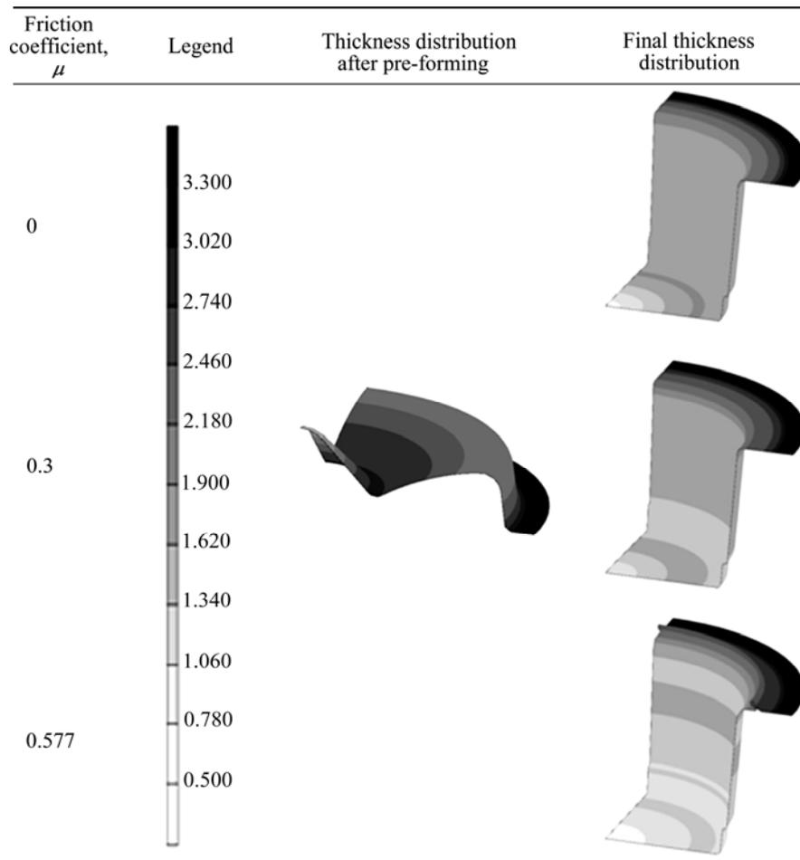
Fig. 5 Final thickness distribution of sidewall of deep cylinder for different friction coefficients of forming die
