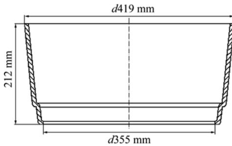
Fig. 1 Geometry of Ti-6Al-4V deep cylinder
