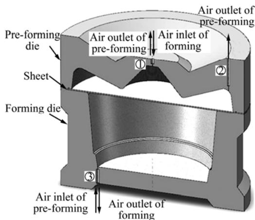
**Fig. 8** Structural diagram of dies used for direct-reverse superplastic forming
