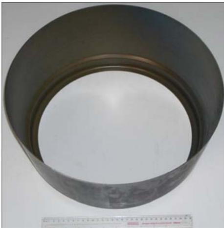
**Fig. 12** Ti–6Al–4V deep cylinder with near uniform thickness distribution
