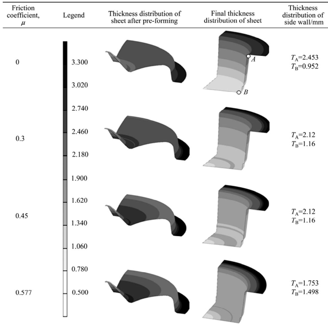
Fig. 4 Final thickness distribution of sidewall of deep cylinder for different friction coefficients of pre-forming die
