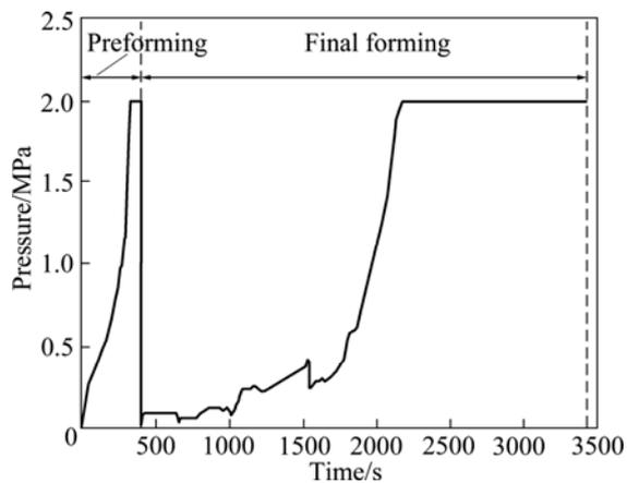
Fig. 6 Time–pressure curve at strain rate of  $0.002 \text{ s}^{-1}$
