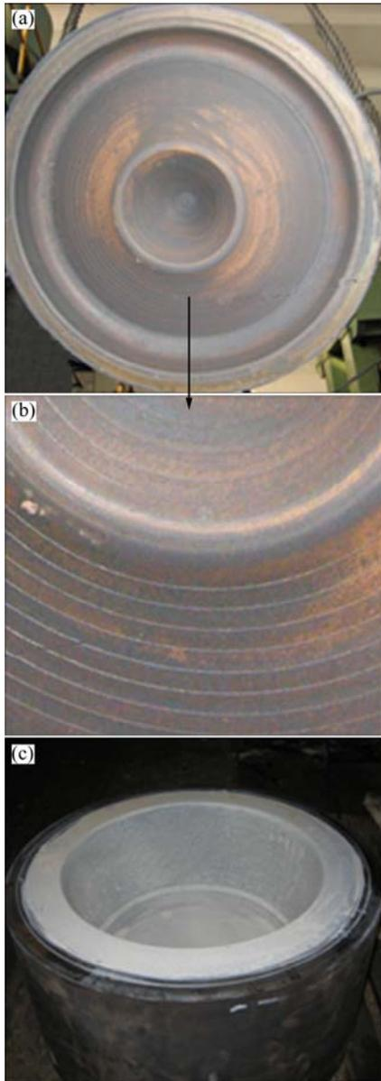
**Fig. 7** Surface of pre-forming die and forming die: (a), (b) Pre-forming die and grooves on surface; (c) Forming die and BN coating on surface
