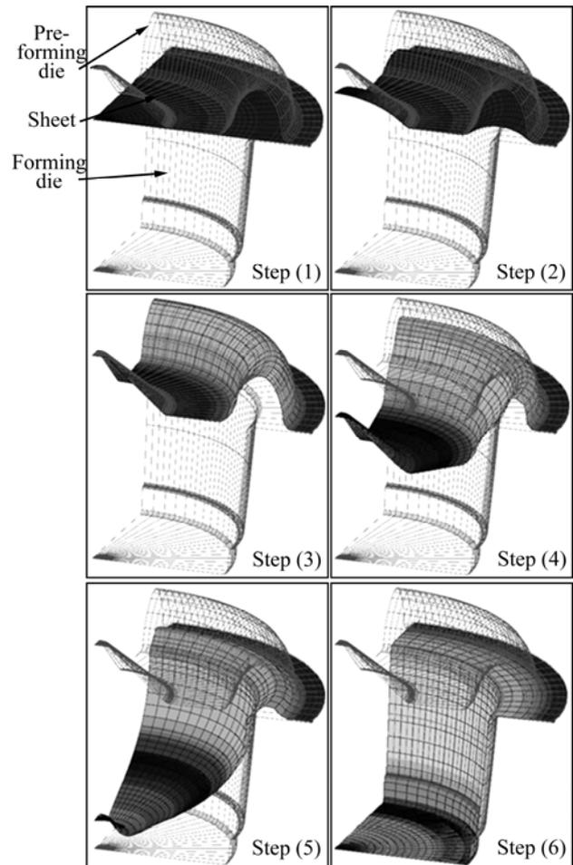
Fig. 2 FEM process of direct-reverse superplastic forming of Ti-6Al-4V deep cylinder
