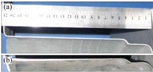
**Fig. 11** Comparison of sectional thickness distribution: (a) Formed by changing friction direct-reverse forming; (b) Formed by common direct-reverse superplastic forming
