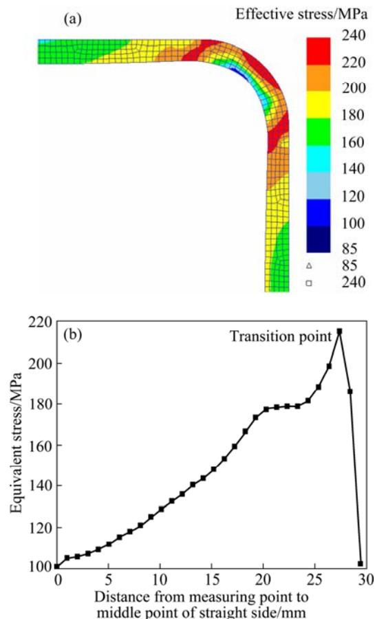
**Fig. 5** Equivalent stress distribution after hydroforming: (a) Numerical simulation on equivalent stress distribution; (b) Equivalent stress distribution of inner face
