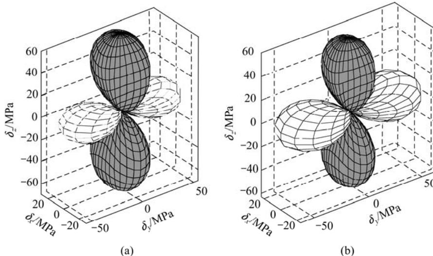
**Fig. 8** Normal stress 3D figures of point Mi (unit: MPa): (a) Total stress (56, -7, -70); (b) Deviator stress (63, 0, -63)
