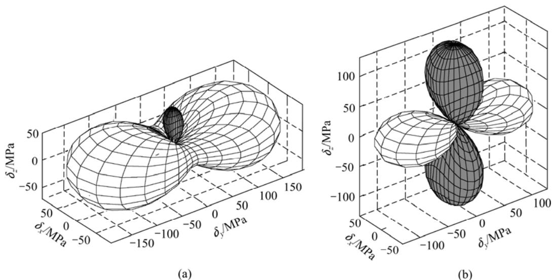
**Fig. 9** Normal stress 3D figures of point Ti (unit: MPa): (a) Total stress (193, 57, -70); (b) Deviator stress (132, 0, -132)
