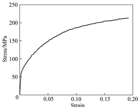
Fig. 2 True stress—strain curve of 5A02 aluminum alloy tube
