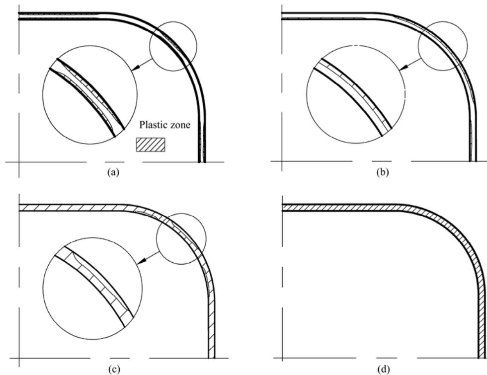
**Fig. 6** Occurrence and development of plastic region: (a) Die closing; (b) Internal pressure of 2.5 MPa ( $0.03\sigma_s$ ); (c) Internal pressure of 7.0 MPa ( $0.09\sigma_s$ ); (d) Internal pressure of 11.0 MPa ( $0.14\sigma_s$ )
