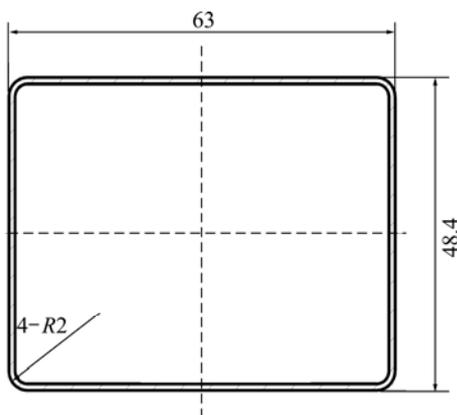
Fig. 1 Shape and dimensions of rectangular section (unit: mm)
