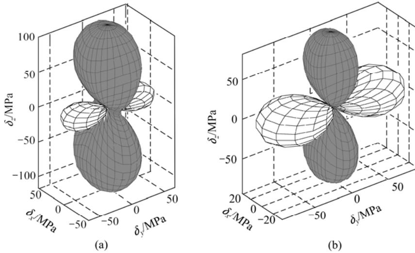
Fig. 10 Normal stress 3D figures of point Ci (unit: MPa): (a) Total stress (69, -24, -118); (b) Deviator stress (93, 0, -93)
