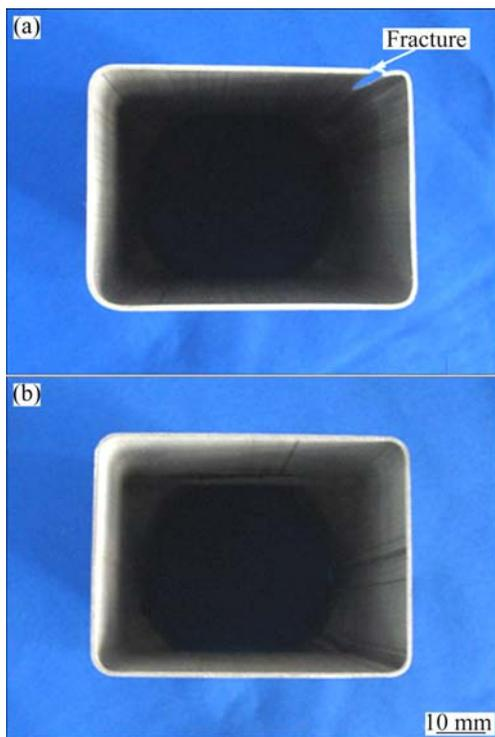
**Fig. 4** Experimental results: (a) Bursting at transition zone; (b) Cross-section shape of final part
