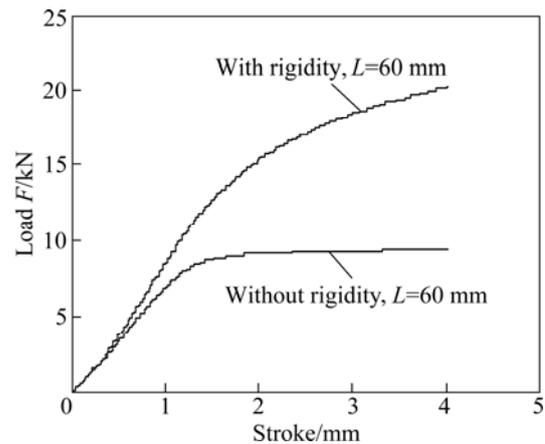
**Fig. 3** Force—stroke curve with and without rigidity
