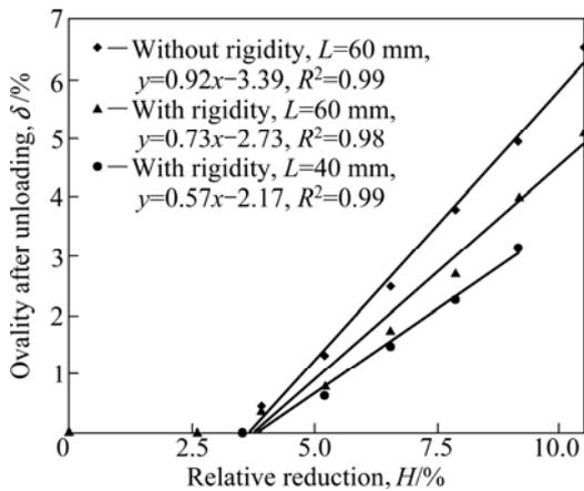
Fig. 4 Curves of ovality after unloading and relative reduction
