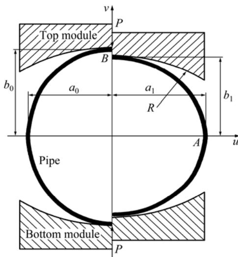
Fig. 1 Sketch of mould press type over-bending setting round
