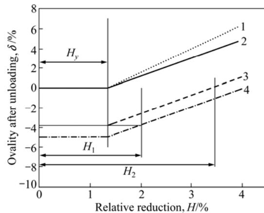
Fig. 5 Sketch of two-step control strategy: 1—Circle-to-oval process for whole pipe; 2—Circle-to-oval process for pipe-end; 3—Setting round process when initial ovality is  $\delta_0$ ; 4—Setting round process when initial ovality is  $\delta_1$
