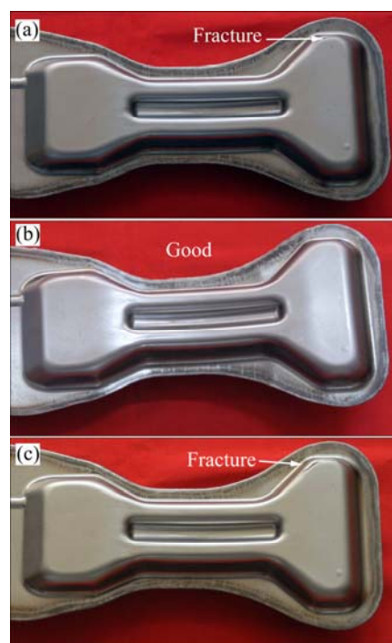
Fig. 9 Parts formed by Path 1(a), Path 2(b) and Path 3(c)
