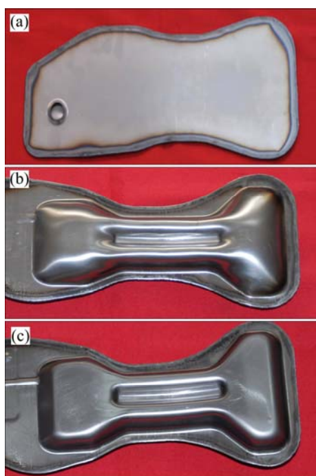
Fig. 4 Forming steps and parts of forming procedure: (a) Welded double sheet; (b) Preforming; (c) Calibrating
