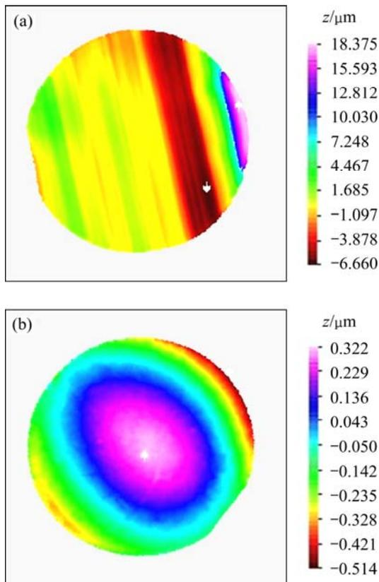
**Fig. 6** Flatness error of sliced (a) and ground with #600 diamond wheel (b) SiC wafers
