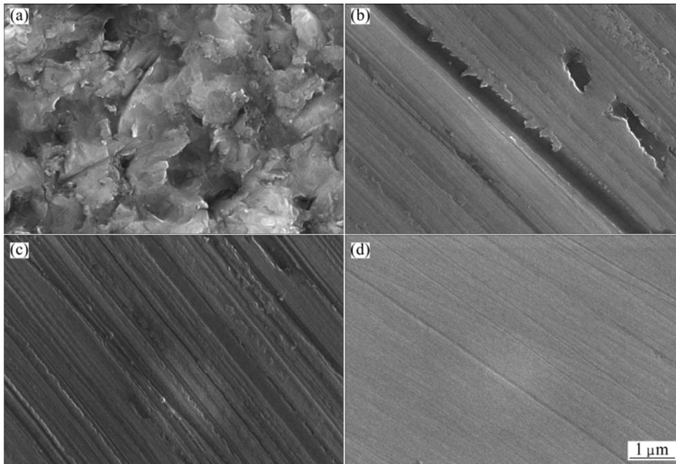
**Fig. 4** SEM images of SiC wafers: (a) Double side lapped; (b) Ground with #600 diamond wheel; (c) Ground with #2000 diamond wheel; (d) Ground with #12000 diamond wheel
