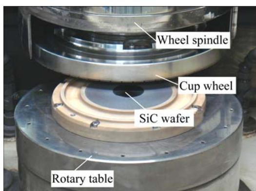
Fig. 1 Photograph of grinding set-up
