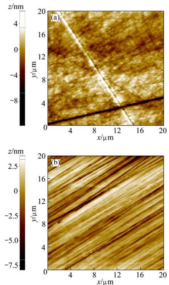
**Fig. 5** AFM micrographs of SiC wafers: (a) Mechanical polished; (b) Ground with #12000 wheel
