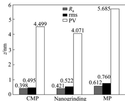
**Fig. 7** Comparison of surface roughness among chemical mechanical polishing (CMP), nanogrinding and mechanical polishing (MP)
