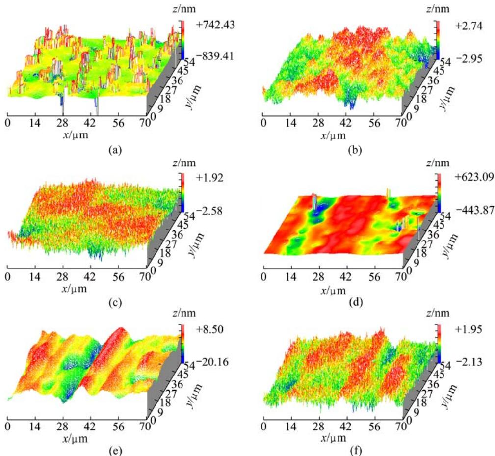
**Fig. 3** Surface topographies of SiC wafers: ((a) Double side polished; (b) Mechanical polished; (c) Chemical mechanical polished; (d) Ground with #600 diamond wheel; (e) Ground with #2000 diamond wheel; (f) Ground with #12000 diamond wheel
