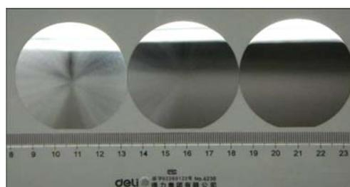
Fig. 2 Photographs of SiC wafers ground with #600, #2000 and #12000 diamond wheels, respectively
