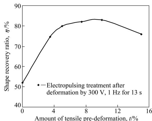
Fig. 1 Effect of amount of tensile pre-deformation on shape recovery ratio
