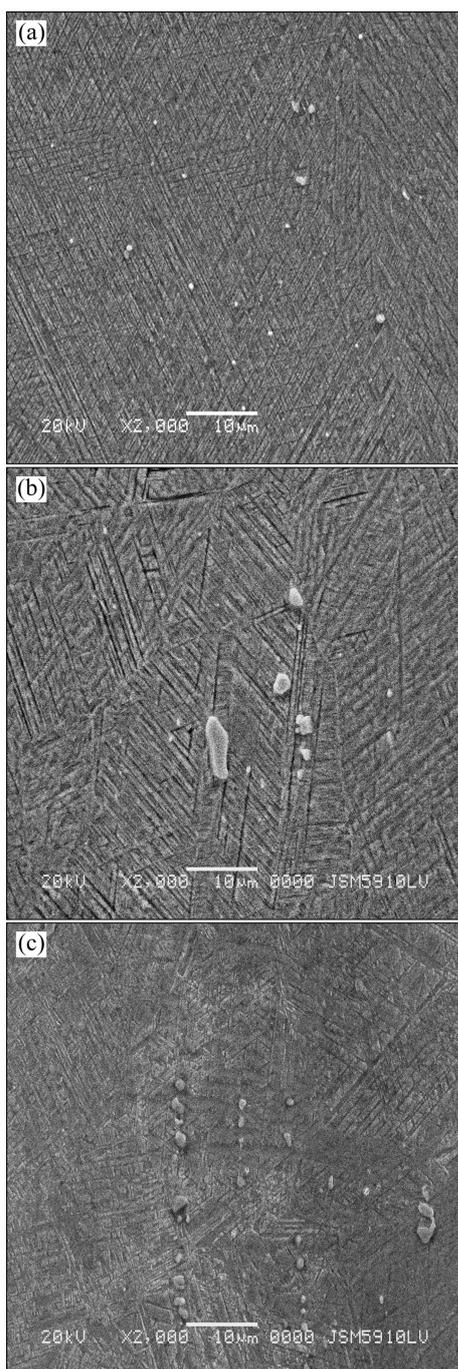
**Fig. 4** SEM images of second phases after 10% pre-deformation by 300 V, 1 Hz electropulsing treatment for 13 s (a), by 300 V, 1 Hz electropulsing treatment for 20 s (b) and by ageing at 1073 K for 1800 s (c)
