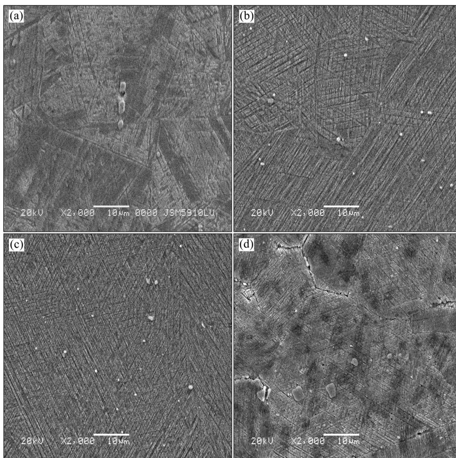
**Fig. 3** SEM images of second phases by 300 V, 1 Hz electropulsing treatment for 13 s after different amounts of pre-deformation: (a) 0; (b) 5%; (c) 10%; (d) 15%
