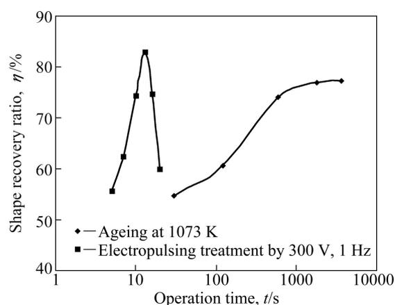
Fig. 2 Effect of operation time on shape recovery ratio of specimens subjected to electropulsing treatment and ageing after 10% pre-deformation
