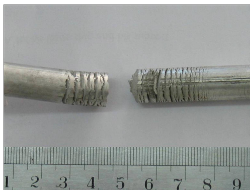
Fig. 4 Cracks and fractures of recycled AZ91D magnesium alloy extruded in 1.2 mm/s at 400 °C
