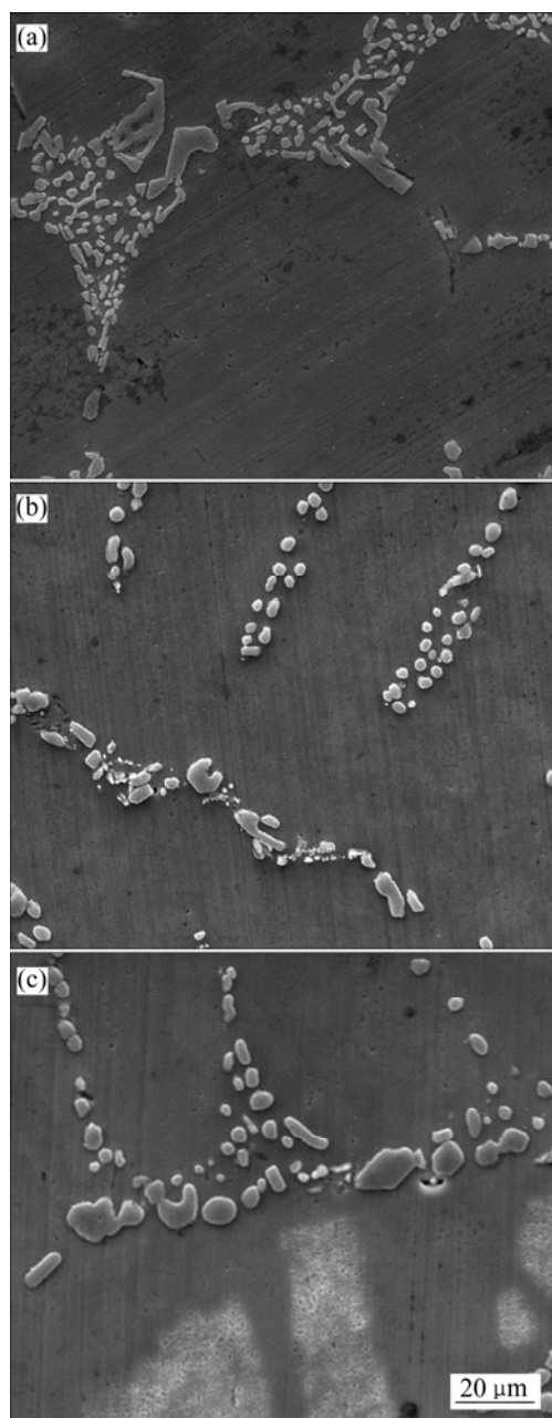
Fig. 5 Morphology of eutectic silicon of A356 aluminum alloy obtained with: (a) as-cast of expendable pattern shell casting; (b) T6 of expendable pattern shell casting; (c) T6 of LFC
