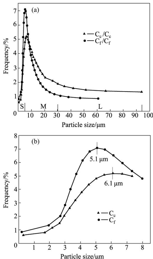
**Fig. 3** Size distributions of wear particles from C/C composites with different preforms in hip joint simulator
