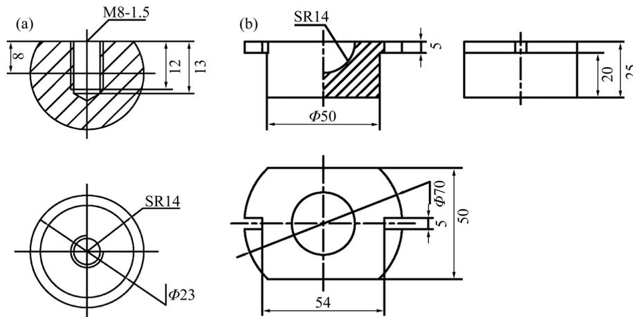
**Fig. 2** Dimensions of femoral head (a) and acetabular cup (b) in hip joint simulator (Unit: mm)
