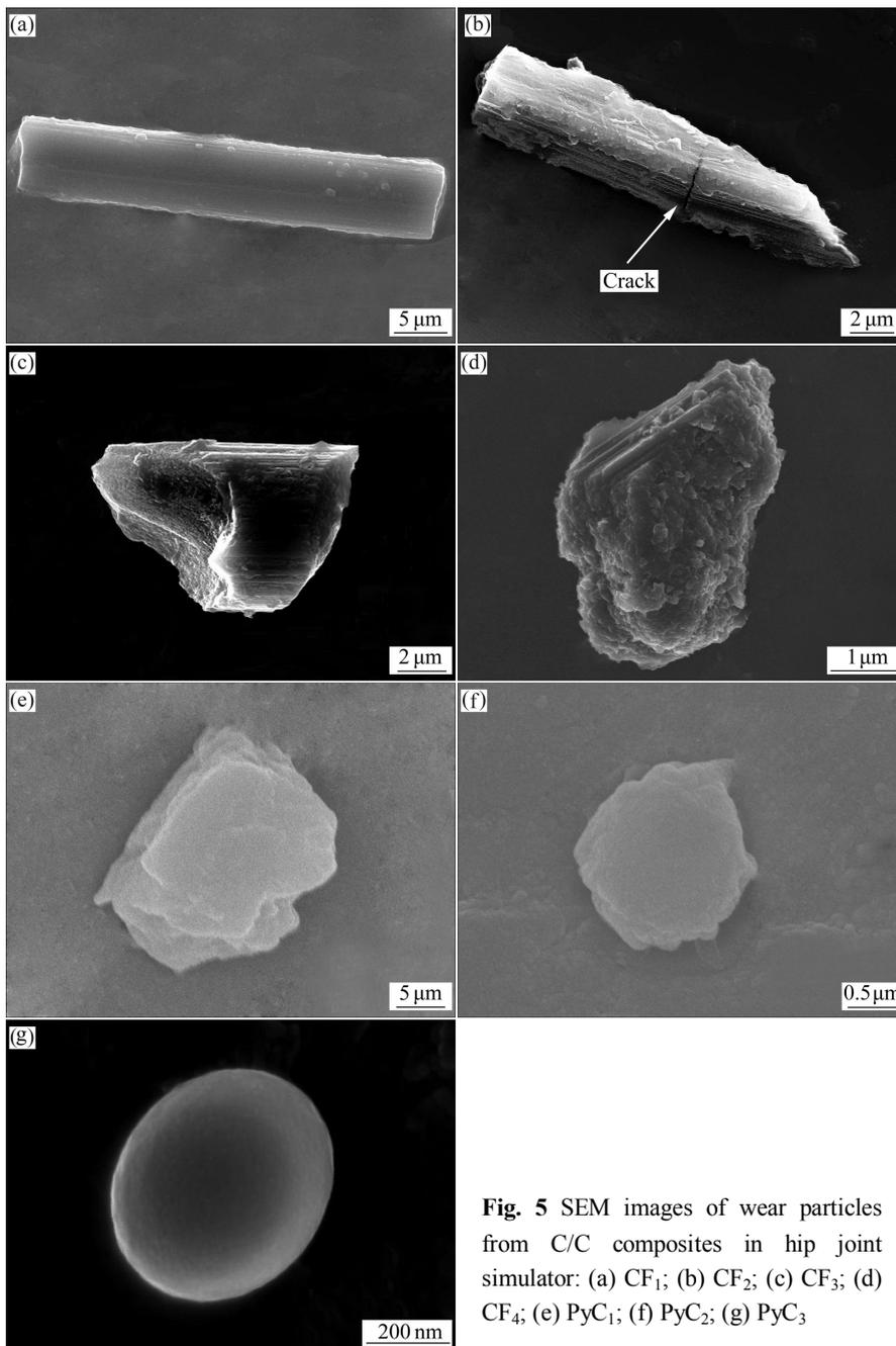
**Fig. 5** SEM images of wear particles from C/C composites in hip joint simulator: (a) CF<sub>1</sub>; (b) CF<sub>2</sub>; (c) CF<sub>3</sub>; (d) CF<sub>4</sub>; (e) PyC<sub>1</sub>; (f) PyC<sub>2</sub>; (g) PyC<sub>3</sub>
