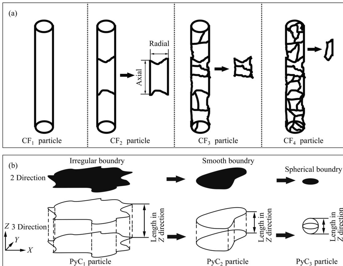
Fig. 6 Evolvement of carbon fiber particles (a) and pyrolytic carbon particles (b) of C/C composites in hip joint simulator
