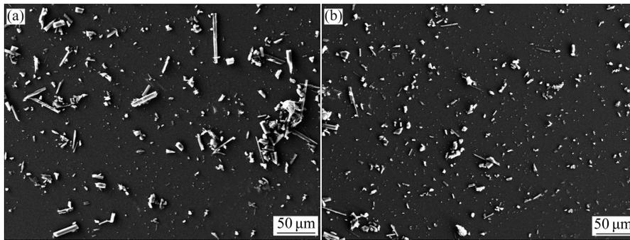
**Fig. 4** SEM images of wear particles from C/C composites with different preforms: (a) Needled carbon cloth preform; (b) Carbon felt preform
