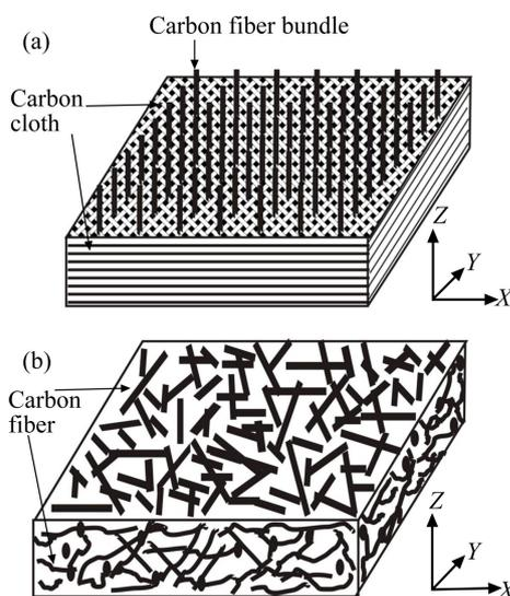
**Fig. 1** Schematic diagrams of preform structures of C/C composites: (a) Needled carbon cloth preform; (b) Carbon felt preform
