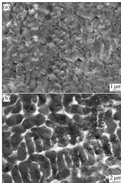
**Fig. 4** High magnification SEM images of ceramic coating: (a) Fully melted region; (b) Liquid-phase sintered region
