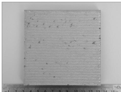
**Fig. 2** Al<sub>2</sub>O<sub>3</sub>–13%TiO<sub>2</sub> ceramic specimen prepared by laser cladding
