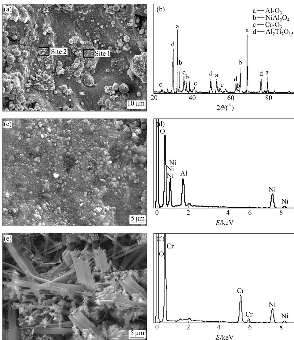
**Fig. 7** SEM morphologies of interface between bond coating and ceramic coating: (a) Overview; (b) XRD pattern; (c) Higher magnification view of site 1; (d) EDS pattern of site 1; (e) Higher magnification view of site 2; (f) EDS pattern of site 2
