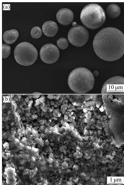
**Fig. 1** SEM images of as-prepared Al<sub>2</sub>O<sub>3</sub>–13%TiO<sub>2</sub> powders: (a) Surface morphology; (b) Cross-sectional structure
