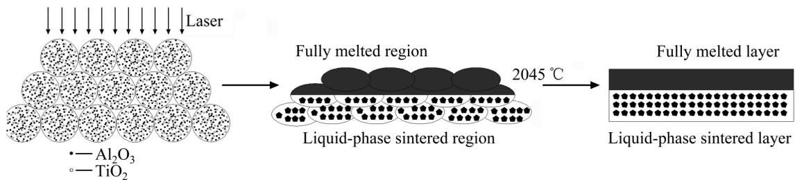
Fig. 6 Schematic illustration of microstructural evolution model indicating evolution of ceramic coating: (a) Early stage; (b) Middle stage; (c) Later stage
