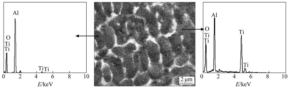
Fig. 5 EDS patterns of liquid-phase sintered region
