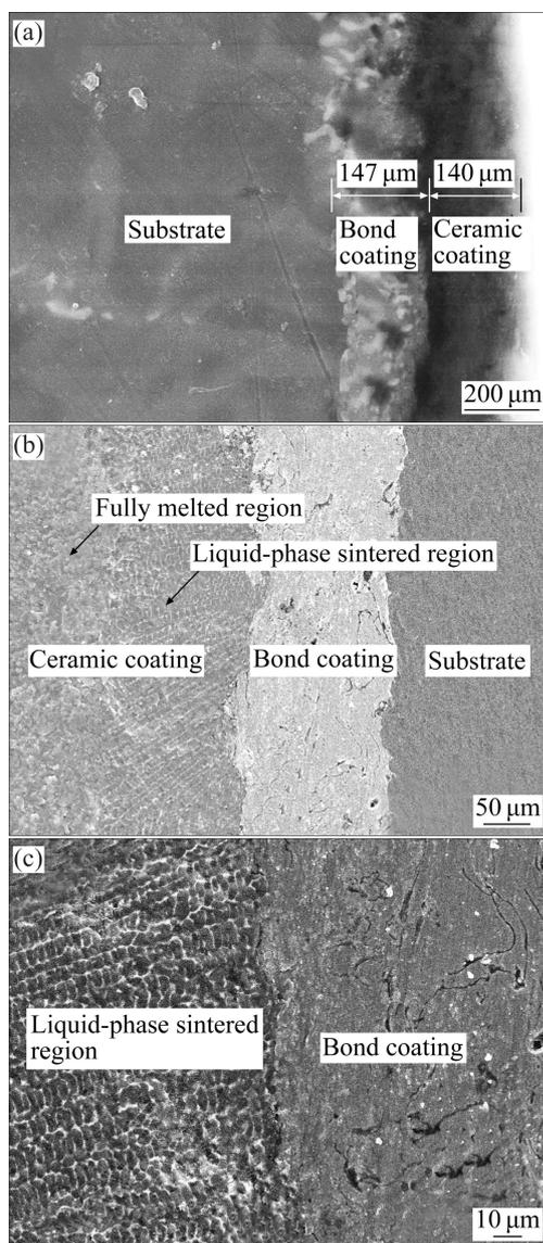
**Fig. 3** Cross-sectional SEM morphologies of laser cladding coating: (a) Overview; (b) High magnification of ceramic coating, bond coating and substrate; (c) High magnification of bond coating and ceramic coating
