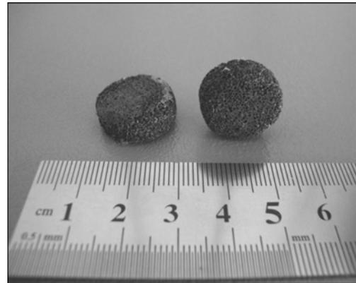
**Fig. 2** Photograph of SiC and B<sub>4</sub>C hybrid preforms
