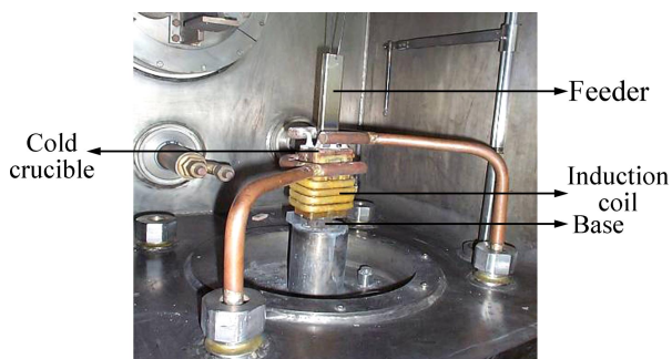
Fig. 1 Photo of rectangular cold crucible system used for continuous melting and DS process
