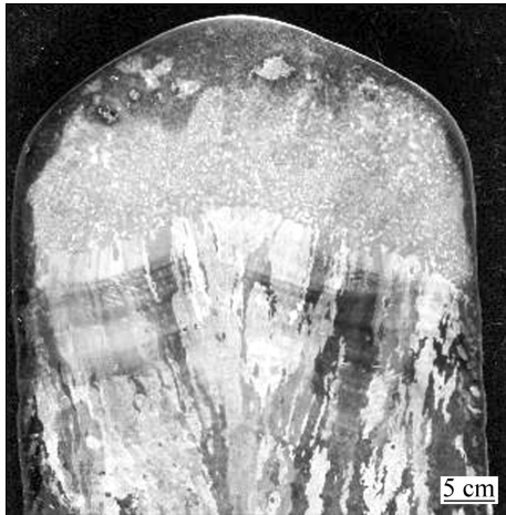
Fig. 3 Photo of S/L interface of Ti–Al ingot directionally solidified by cold crucible
