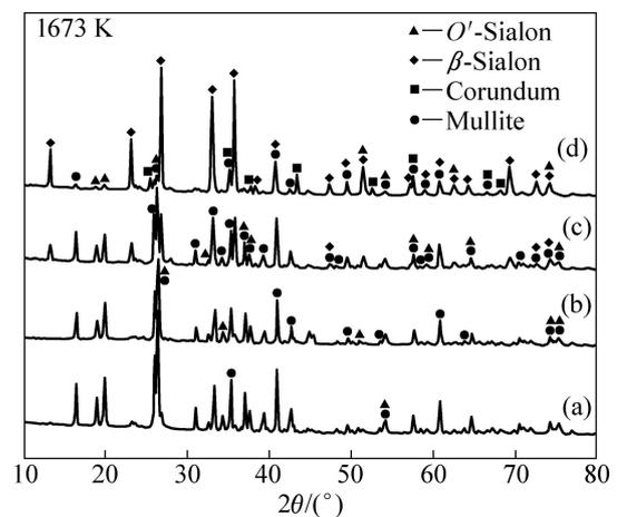
Fig. 2 XRD patterns of samples with different  $m_c/m_f$  values synthesized at 1673 K for 6 h: (a) 0.28; (b) 0.30; (c) 0.42; (d) 0.56
