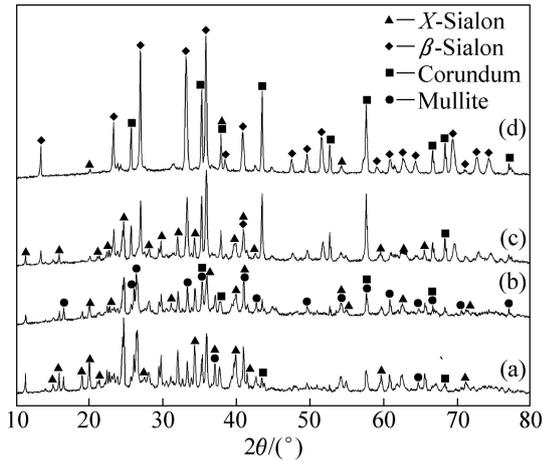
**Fig. 3** XRD patterns of samples with different  $m_c/m_f$  values synthesized at 1723 K for 6 h: (a) 0.28; (b) 0.30; (c) 0.42; (d) 0.56
