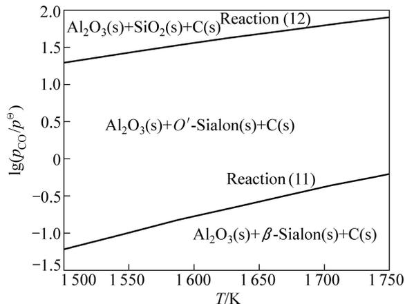
**Fig. 5** Predomination region diagram for  $\text{Al}_2\text{O}_3\text{-SiO}_2\text{-C-N}_2$  system ( $p_{\text{N}_2}=0.1\text{ MPa}$ )
