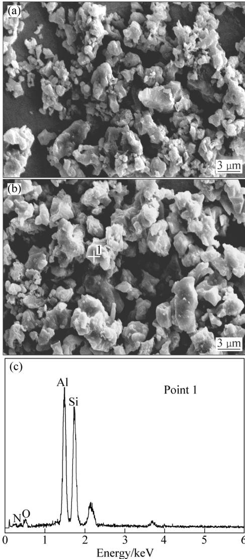
**Fig. 4** SEM images of samples with  $m_c/m_f$  of 0.56 synthesized at 1673 K (a) and 1723 K (b), and EDS pattern of point 1 in Fig. 4(b)
