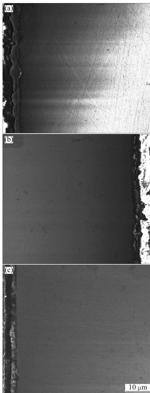
**Fig. 3** Cross-sectional morphologies of pre-oxidized Ni-16Cr-*x*Al alloys: (a) Ni-16Cr-4.5Al alloy; (b) Ni-16Cr-6.8Al alloy; (c) Ni-16Cr-9.0Al alloy
