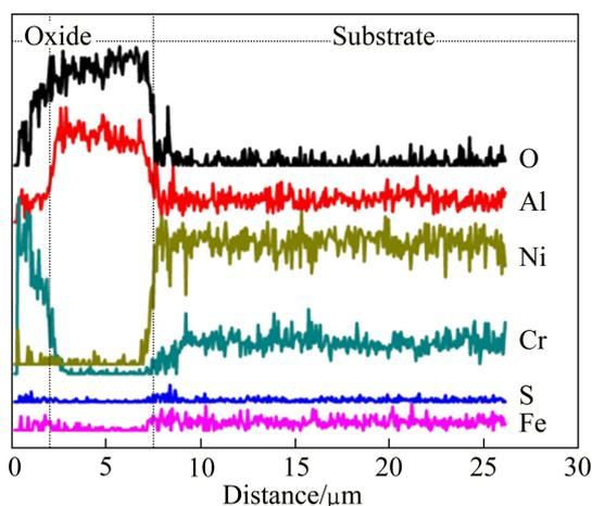
**Fig. 7** Element distribution along arrow marked in Fig. 4(c) after corrosion for 100 h in  $\text{Na}_2\text{SO}_4$ –25% NaCl at  $600\ ^\circ\text{C}$
