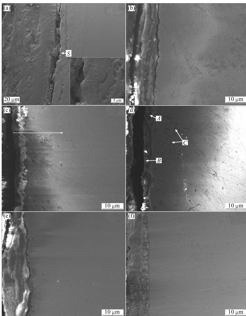
**Fig. 4** Cross-sections of as-cast samples (a, b and c) and pre-oxidized samples (d, e and f) corroded for 100 h in  $\text{Na}_2\text{SO}_4$ -25% NaCl salts at 600 °C: (a), (b), (c) As-cast alloys with Al contents of 4.5%, 6.8%, 9.0%, respectively; (d), (e), (f) Pre-oxidized alloys with Al contents of 4.5%, 6.8%, 9.0%, respectively
