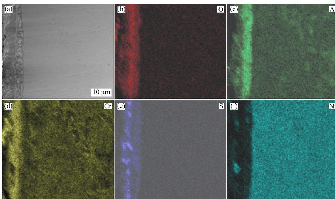
**Fig. 9** Cross-sectional SEM image (a) and corresponding elements mapping (b, c, d, e, f) of pre-oxidized Ni-16Cr-9.0Al after corrosion for 100 h in Na<sub>2</sub>SO<sub>4</sub>-25% NaCl at 600 °C
