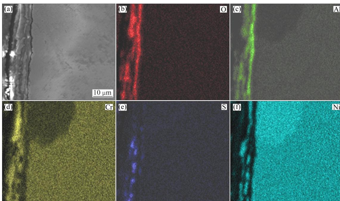
**Fig. 6** Cross-sectional SEM image (a) and corresponding elements mapping (b, c, d, e, f) of as-cast Ni–16Cr–6.8Al after corrosion for 100 h in  $\text{Na}_2\text{SO}_4$ –25% NaCl at 600  $^\circ\text{C}$
