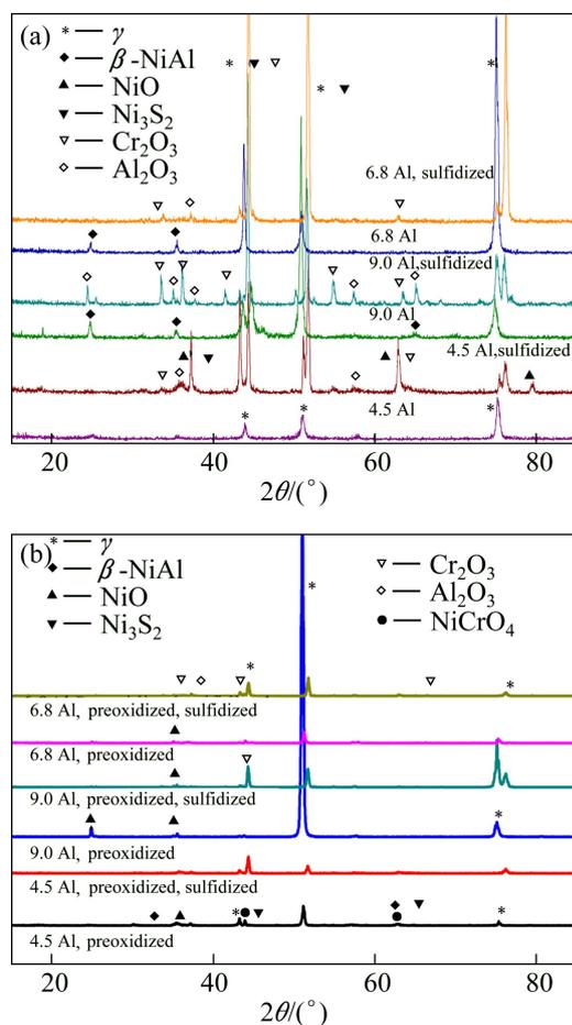
**Fig. 2** XRD patterns of as-cast (a) and pre-oxidized (b) Ni-16Cr-*x*Al alloys before and after hot corrosion for 100 h at 600 °C
