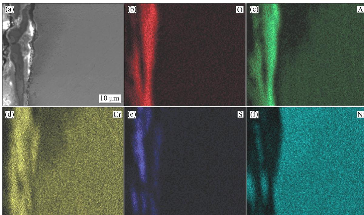
**Fig. 8** Cross-sectional SEM image (a) and corresponding elements mapping (b, c, d, e, f) of pre-oxidized Ni–16Cr–6.8Al after corrosion for 100 h in  $\text{Na}_2\text{SO}_4$ –25% NaCl at  $600\ ^\circ\text{C}$
