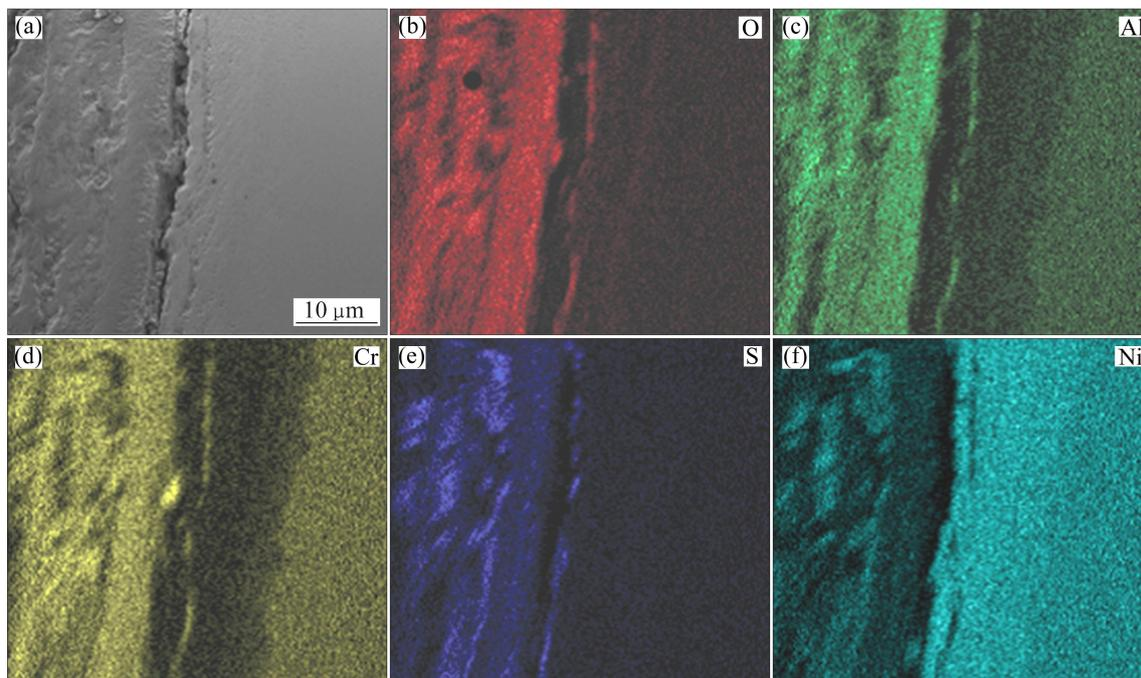
**Fig. 5** Cross-sectional SEM image (a) and corresponding elements mapping (b, c, d, e, f) of as-cast Ni–16Cr–4.5Al after corrosion for 100 h in  $\text{Na}_2\text{SO}_4$ –25% NaCl at 600  $^\circ\text{C}$
