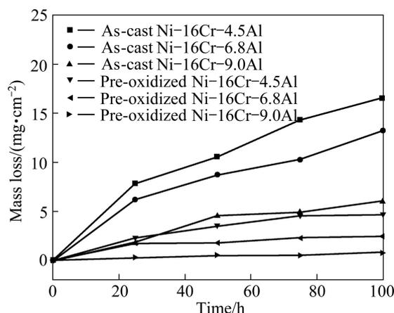
**Fig. 1** Mass change per unit area of pre-oxidized and as-cast specimens as function of time in Na<sub>2</sub>SO<sub>4</sub>–25% NaCl salts at 600 °C
