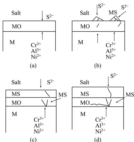
**Fig. 10** Schematic diagram showing growth of sulfide layer on pre-oxidized Ni–16Cr–xAl alloys during hot corrosion in  $\text{Na}_2\text{SO}_4$ –25% NaCl at 600 °C: (a) Diffusion of  $\text{S}^{2-}$ ,  $\text{Al}^{3+}$ ,  $\text{Cr}^{3+}$  and  $\text{Ni}^{2+}$  in oxide layer; (b) Nucleation of sulfides at oxide/salt interface; (c) Formation of sulfides in oxide layer; (d) Growth of sulfides near oxide/alloy interface
