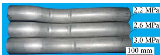
Fig. 5 Bent tube under different pressures (plan 1)
