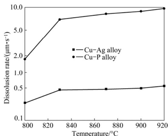
Fig. 4 Dissolution rate of Cu in Cu–P and Cu–Ag alloys in temperature range of weld brazing
