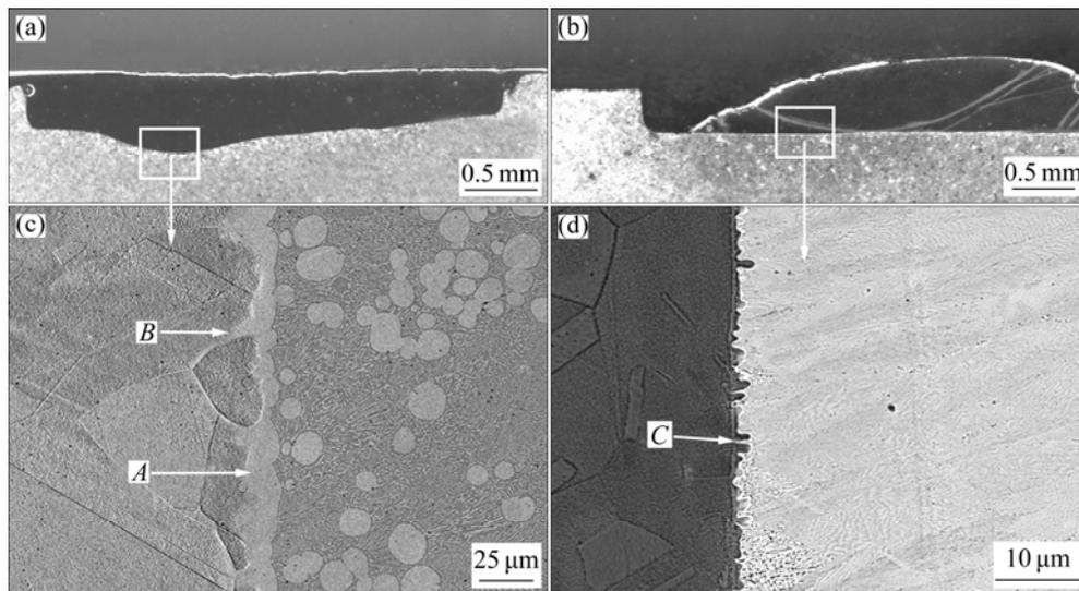
**Fig. 5** Macrostructure and microstructure of interface using arc heating: (a), (c) Cu–P alloys; (b), (d) Cu–Ag alloys
