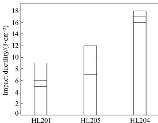
**Fig. 7** Impact ductility of welding joints with different filler metals
