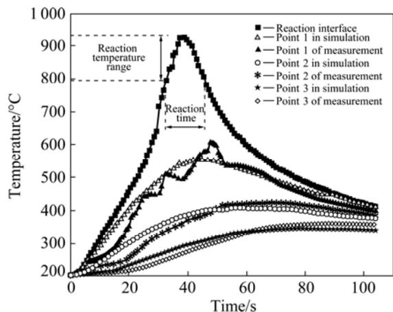
**Fig. 3** Thermal cycle curves at reaction interface during one thermal cycle
