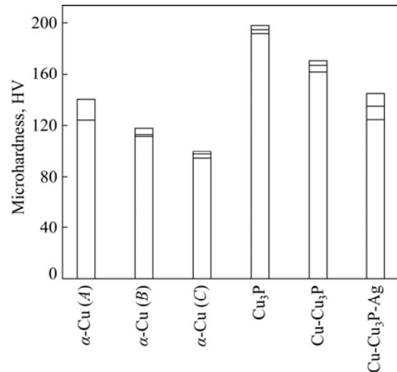
**Fig. 8** Micro-hardness of different phases in welds
