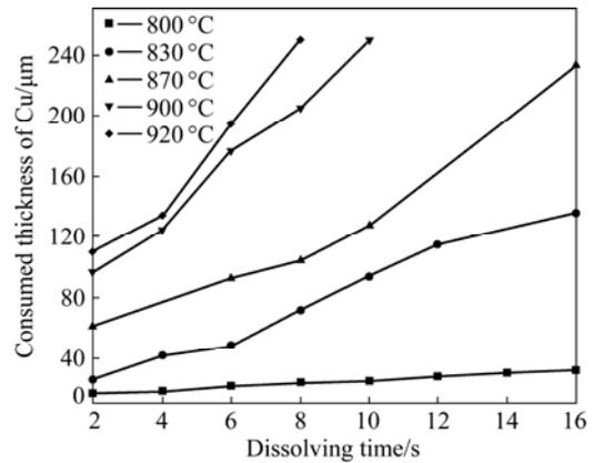
**Fig. 1** Consumed thickness of Cu in Cu–P alloys at different temperatures for different time
