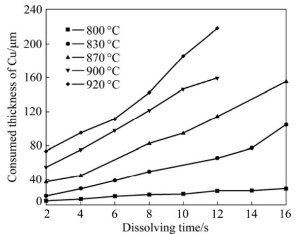
**Fig. 2** Consumed thickness of Cu in Cu–Ag alloys at different temperatures for different time
