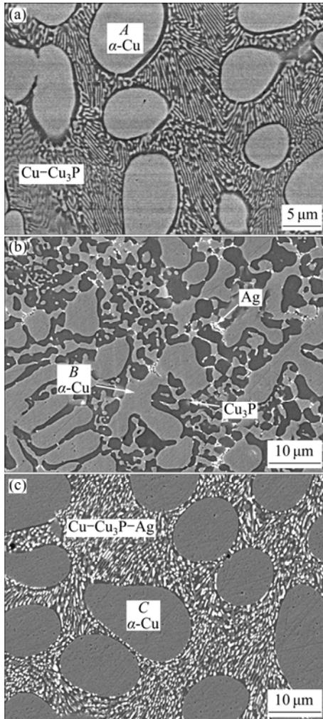
**Fig. 6** Backscattered electron images of welds with different filler metals: (a) HL201; (b) HL205; (c) HL204
