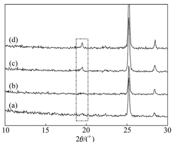
**Fig. 4** XRD patterns of 55% Euc/Al composites with different stress relief annealing time at 190 °C: (a) 0 h; (b) 3 h; (c) 6 h; (d) 9 h
