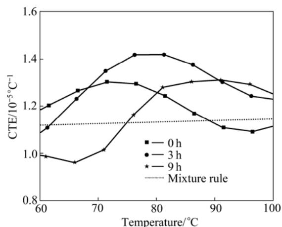
**Fig. 5** CTE curves of 55% Euc/Al composites with different stress relief annealing time at 190 °C
