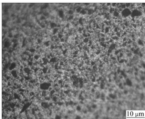
Fig. 1 OM micrograph of 35% Euc/Al composite
