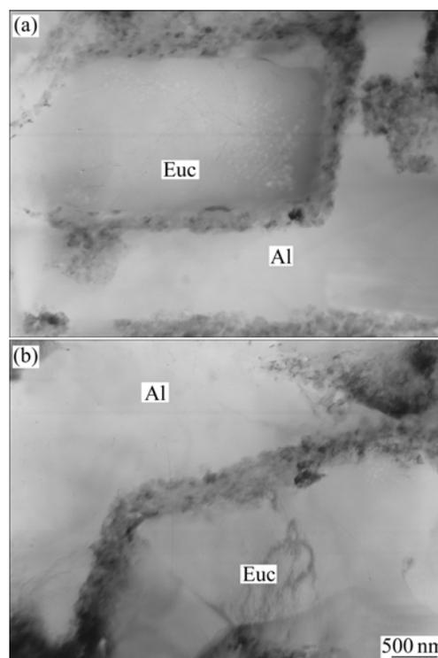
Fig. 2 TEM images of Euc/Al composites: (a) As-sintered composite; (b) Composite heated at 500  $^{\circ}\text{C}$  for 3 h
