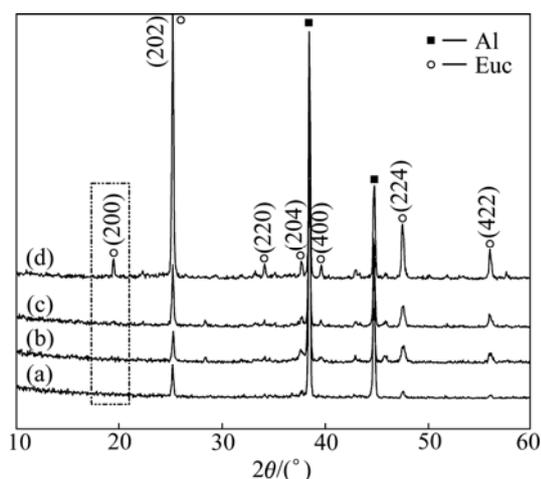
**Fig. 3** XRD patterns of Euc/Al composites with different volume fractions of  $\beta$ -eucryptite: (a) 15% Euc/Al; (b) 35% Euc/Al; (c) 55% Euc/Al; (d) 75% Euc/Al
