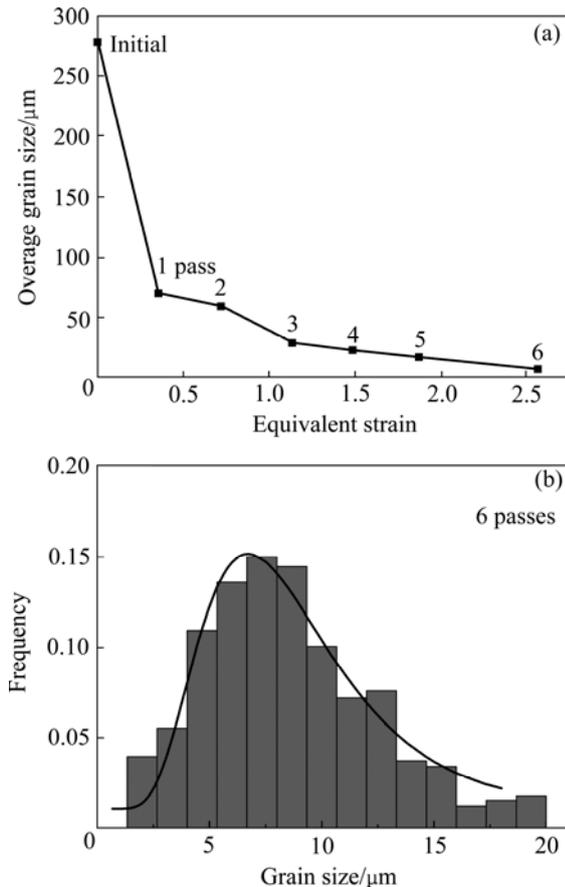
**Fig. 4** (a) Average grain size of as-rolled ZK60 Mg alloy after different rolling passes; (b) Grain size distribution of ZK60-HR (6 passes)
