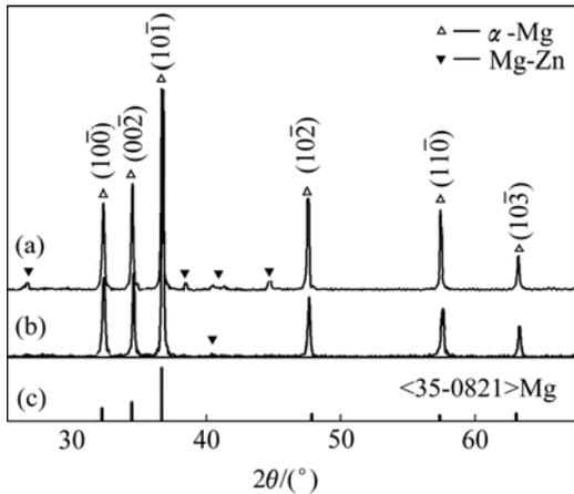
**Fig. 1** XRD patterns of ZK60-C (a), ZK60-ST (b) and magnesium standard card (c)
