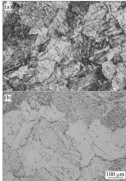
**Fig.2** Microstructures of ZK60-C (a) and ZK60-ST (b) alloy billet
