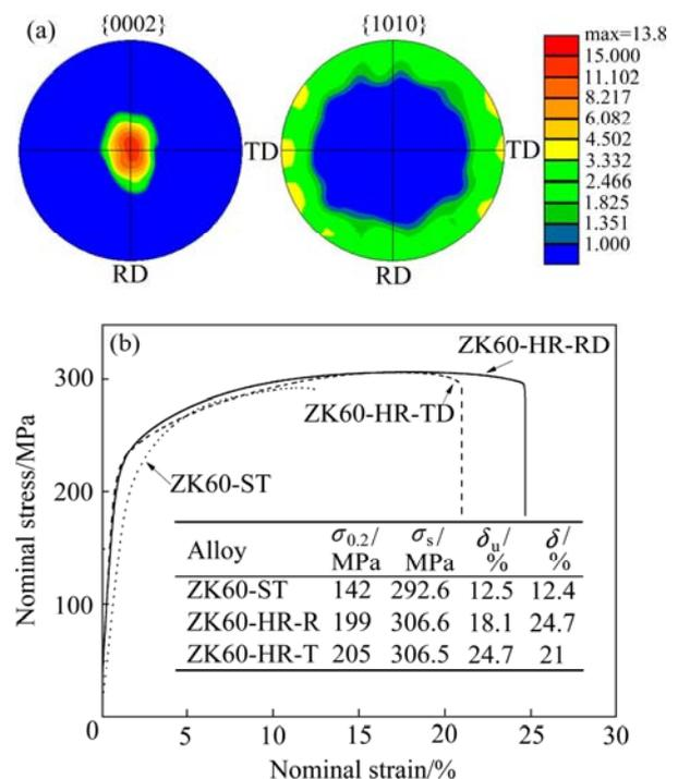
**Fig. 5**  $\{0001\}$  and  $\{10\bar{1}0\}$  pole figures of ZK60-HR (a) and stress—strain curves of ZK60-ST and ZK60-HR (b)
