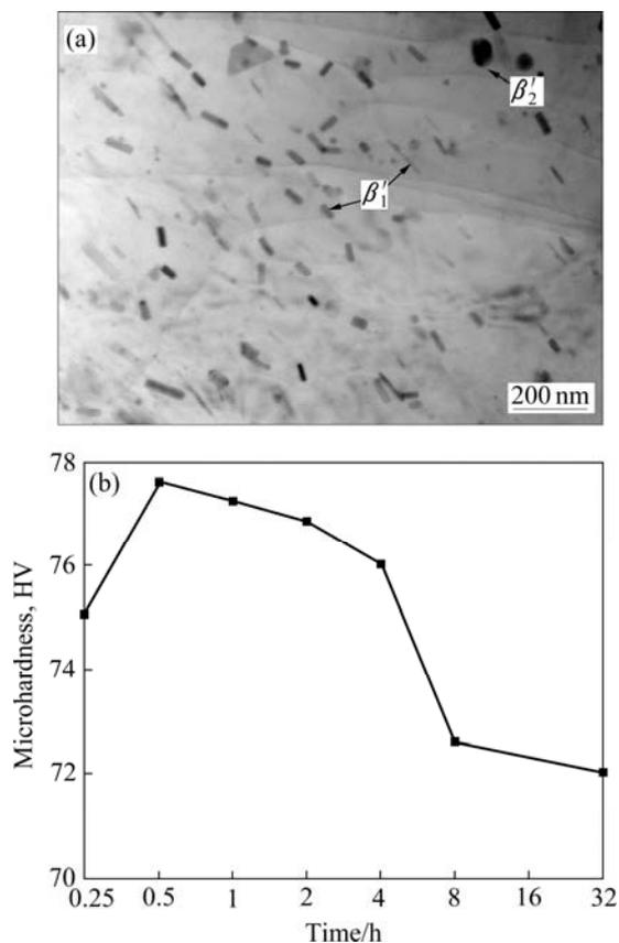
**Fig. 6** TEM image (a) and micro-hardness (b) curve of ZK60-HR for aging at 175 °C
