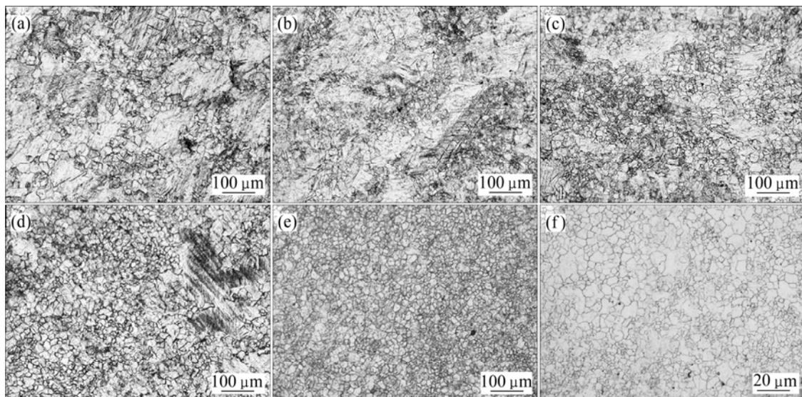
**Fig. 3** Microstructures of as-rolled ZK60 Mg alloy after different rolling passes: (a) 1 pass; (b) 2 passes; (c) 3 passes; (d) 4 passes; (e) 5 passes; (f) 6 passes
