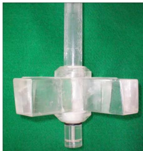
Fig. 2 Photo of four-blade impeller and four-hole nozzle
