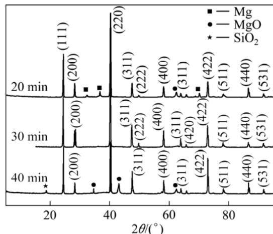
**Fig. 4** XRD patterns of  $\text{Mg}_2\text{Si}$  samples with different holding time during synthesis processing
