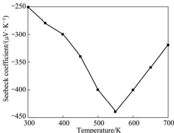
Fig. 6 Variation of Seebeck coefficient with holding temperature for  $\text{Mg}_2\text{Si}$  compounds
