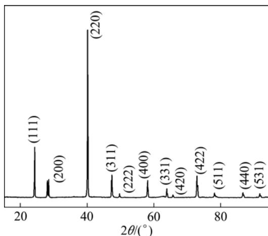
**Fig. 2** XRD pattern of  $\text{Mg}_2\text{Si}$  sample sintered at microwave power of 2.5 kW
