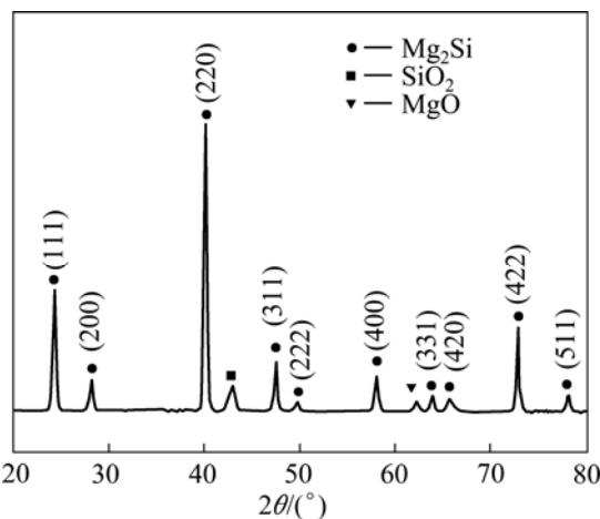
**Fig. 3** XRD pattern of  $\text{Mg}_2\text{Si}$  sample sintered at microwave power of 3.5 kW
