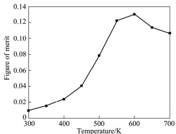
Fig. 8 Temperature dependency of figure of merit,  $ZT$ , for  $\text{Mg}_2\text{Si}$  compound
