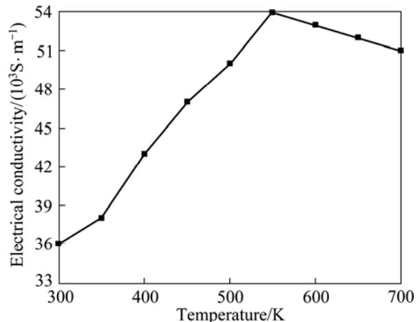
**Fig. 5** Variation of electrical conductivity with holding temperature for  $\text{Mg}_2\text{Si}$  compounds
