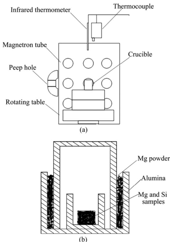
**Fig. 1** Schematic diagrams of microwave system setup (a) and crucible (b)
