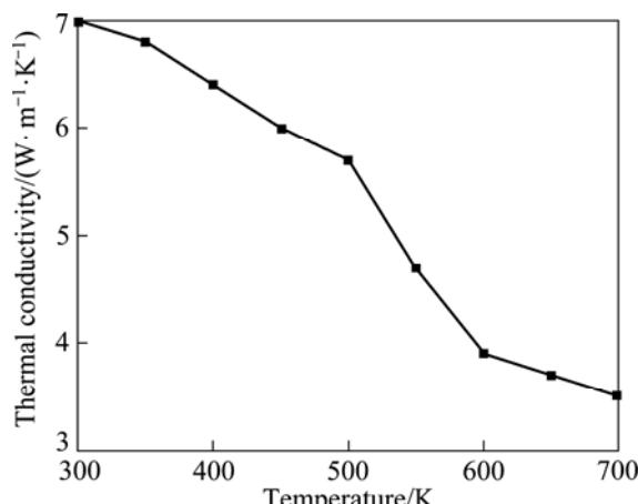
Fig. 7 Variation of thermal conductivity with holding temperature for  $\text{Mg}_2\text{Si}$  compound
