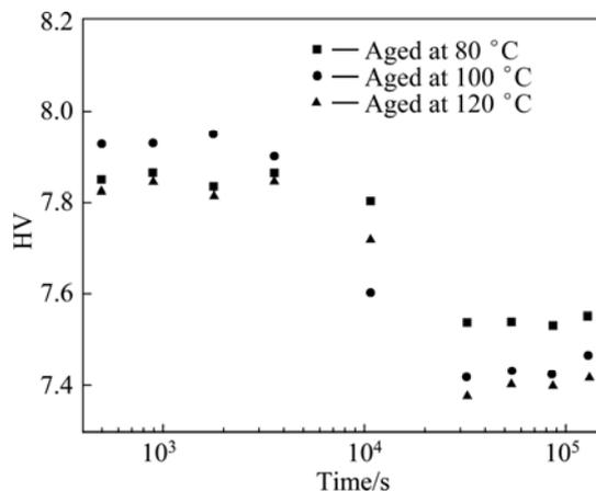
**Fig. 8** Evolution of Vickers hardness versus isothermal annealing time of Pb-0.08Ca-2Sn samples cold rolled to thickness reduction of 70%
