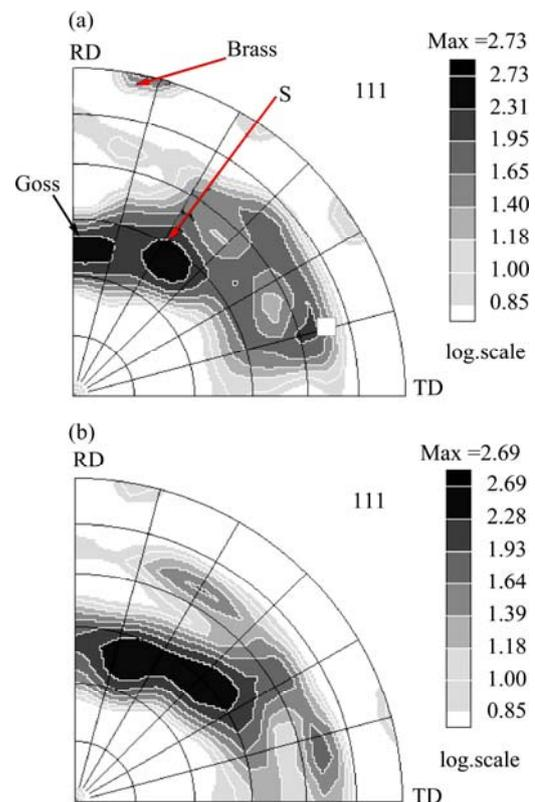
**Fig. 2**  $\{111\}$  pole figures of cold rolled Pb-0.08Ca-2Sn samples to thickness reduction of 50% (a) and 75% (b) (White filled square represents  $\{\bar{2}11\}\langle 011\rangle$  shearing texture component)
