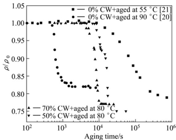
**Fig. 7** Evolution of relative resistivity versus isothermal annealing time of cold rolled Pb-0.08Ca-2Sn samples (Results in Refs. [20] and [21] are given for comparison)
