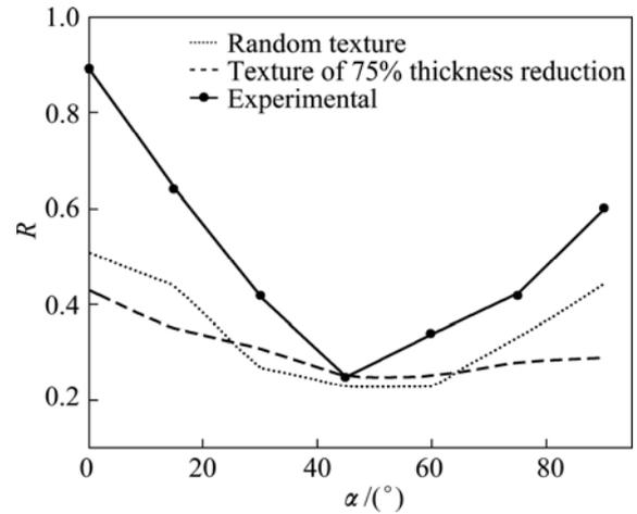
**Fig. 4** Evolution of planar Lankford anisotropy or  $R$  value versus angle ( $\alpha$ ) to rolling direction for Pb-0.08Ca-2Sn samples cold rolled to a thickness reduction of 70% (Dotted and dashed lines represent plots of  $R$  value calculated using texture data with random and that of experimental pole figures)
