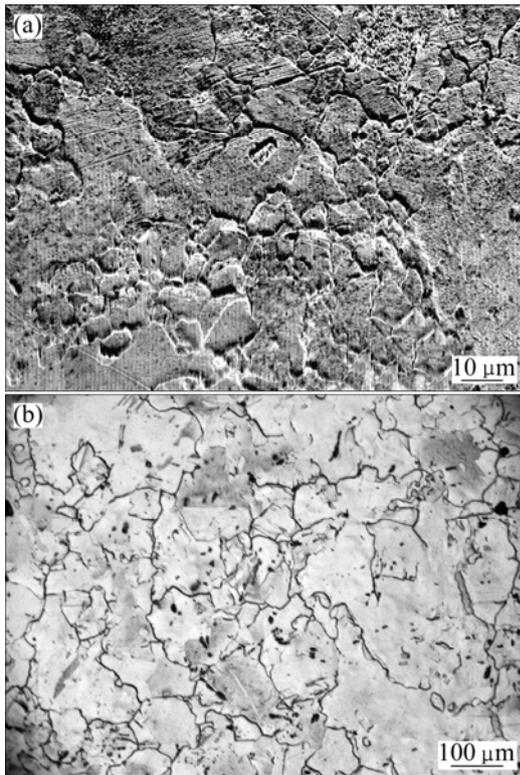
**Fig. 5** SEM micrographs showing features of recrystallization of cold rolled Pb-0.08Ca-2Sn alloys: (a) Annealed at 100 °C for 1 h; (b) Annealed at 100 °C for 6 h
