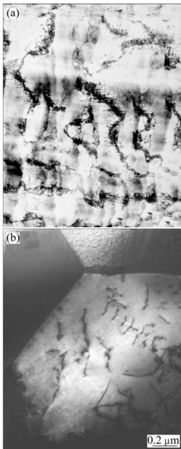
**Fig. 1** TEM micrographs showing typical elements of defects in deformed Pb-0.08Ca-2Sn alloy: (a) Dislocation networks on sub-boundaries; (b) Micro-slip lines
