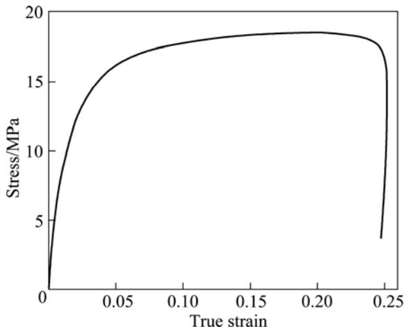
**Fig. 3** Stress—strain plot for Pb-0.08Ca-2Sn alloy cold rolled to a thickness reduction of 75% with strain rate of  $2 \times 10^{-4} \text{ s}^{-1}$
