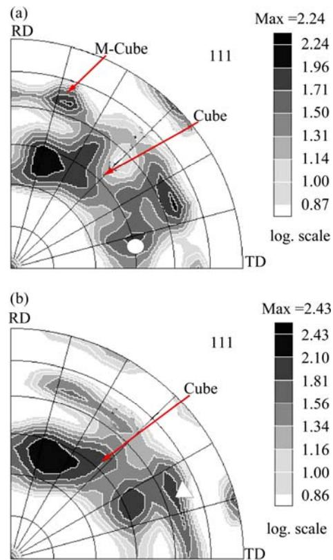
**Fig. 6**  $\{111\}$  pole figures of cold rolled Pb-0.08Ca-2Sn samples with thickness reduction of 50% (a) and 75% (b) (White filled circle and triangle represent the Sh1  $\{1\bar{1}4\}\langle 1\bar{3}1 \rangle$  and Sh2  $\{1\bar{1}\bar{1}\}\langle \bar{1}21 \rangle$  shearing texture components, respectively)
