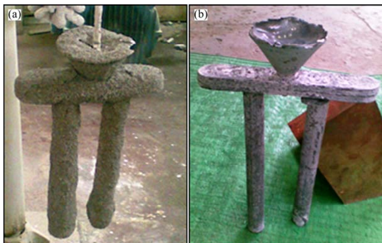
Fig. 1 Cast cp-Ti bars by investment casting: (a) Ceramic mould; (b) Cast bars
