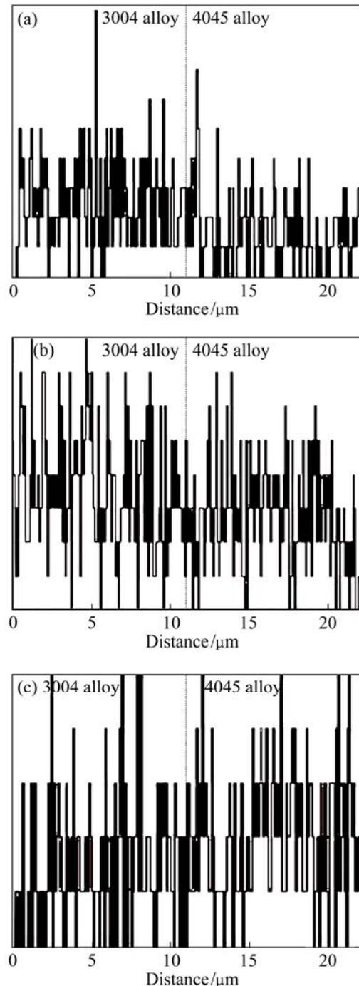
**Fig. 4** Distributions of manganese (a), magnesium (b) and silicon (c) across composite interface
