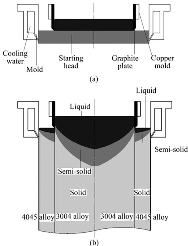
**Fig. 1** Schematic diagrams of casting process at initial (a) and steady (b) states
