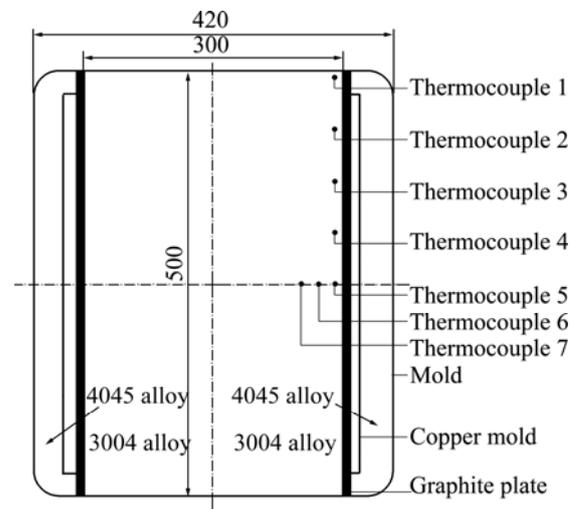
**Fig. 2** Schematic diagram of thermocouple positions (top view)
