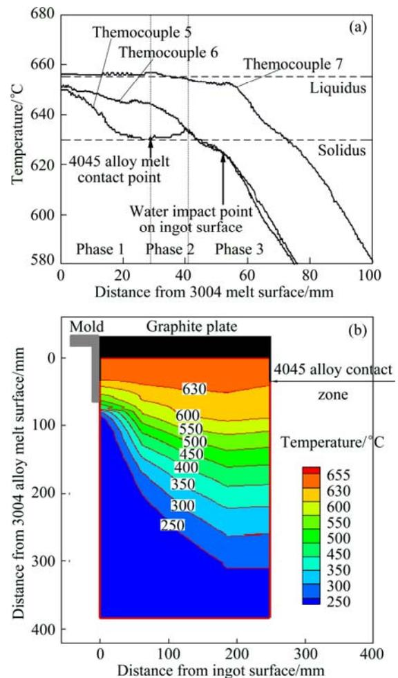
Fig. 7 Cooling curves of thermocouples 5, 6 and 7 (a) and temperature profile of composite interface during casting process (b)
