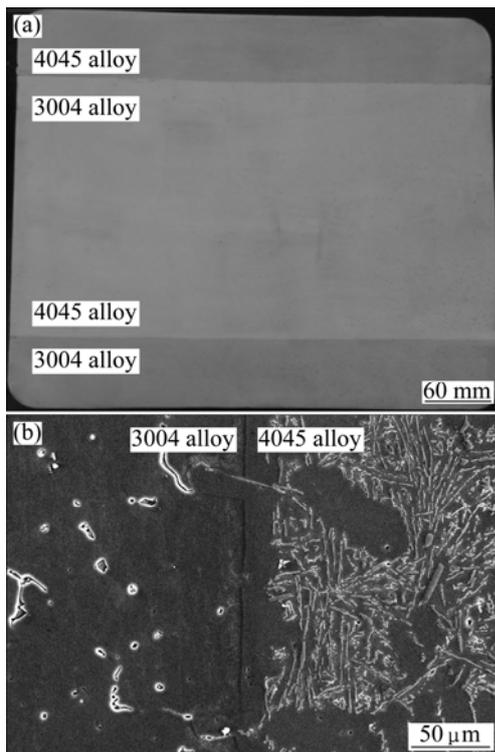
**Fig. 3** Macrostructure (a) and microstructure (b) in cross section of composite ingot
