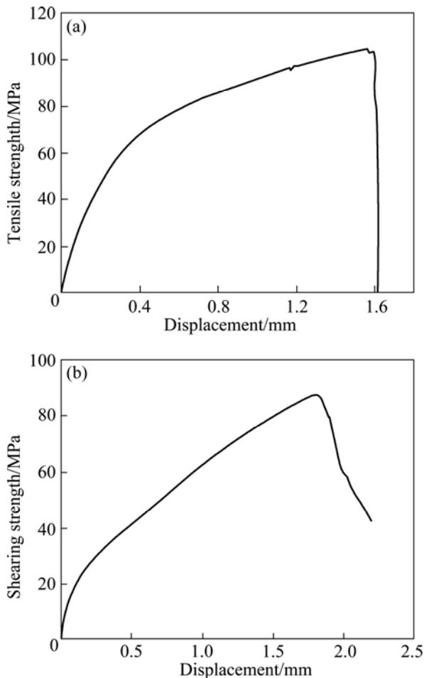
Fig. 6 Tensile strength—displacement (a) and shearing strength—displacement (b) curves of composite ingot
