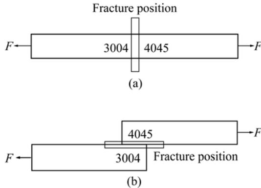
Fig. 5 Schematic diagrams of tensile (a) and shearing (b) tests
