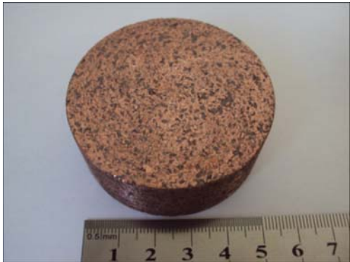
图 3 烧结成型的石墨/铜基复合材料样品 Fig. 3 Sample of sintered graphite/copper based composites
