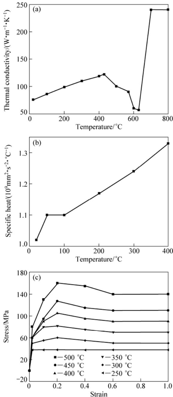
**Fig.2** Properties of AZ31 alloy: (a) Thermal conductivity[14]; (b) Specific heat capacity[14]; (c) Flow stress curves at various temperatures[15]
