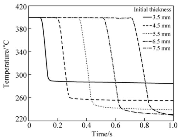
**Fig.4** Temperature curves at different places of sheet with different initial thicknesses
