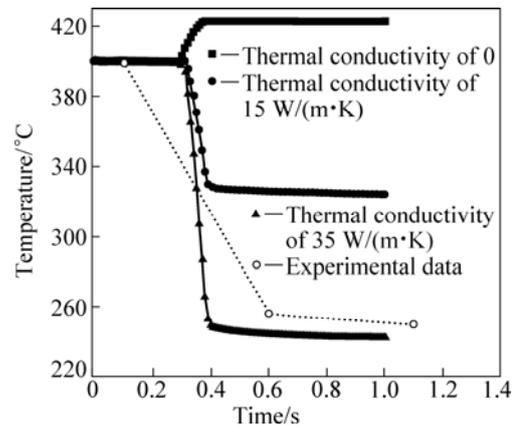
**Fig.3** Temperature curves with different thermal conductivities obtained from FEM and experiment
