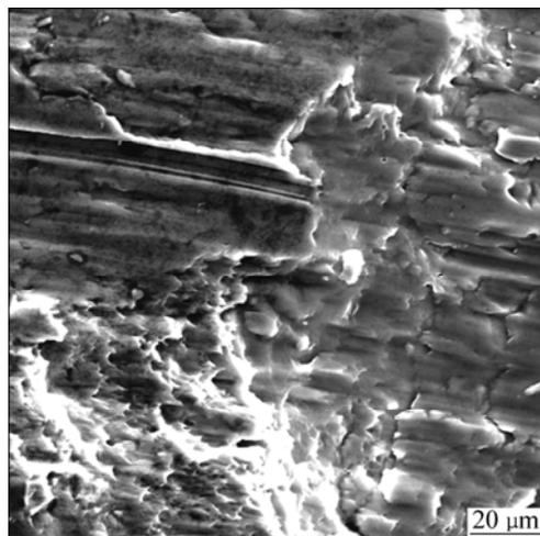
**Fig.7** SEM photo of edge cracks
