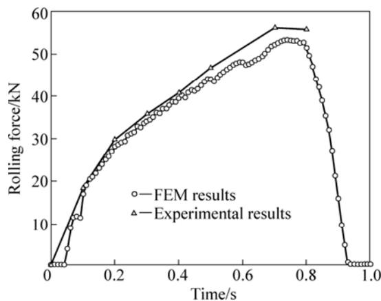
Fig.8 Rolling force curves of experimental and FEM results
