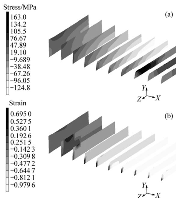
**Fig.6** Map of maximum tensile principal stress (a) and map of major principal plastic strain (b)
