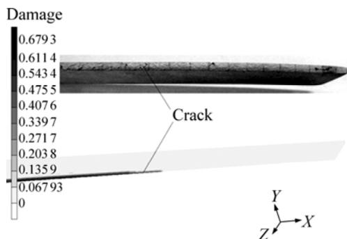
**Fig.5** Edge crack results of experiment and FEM (Holes in edge of sheet are location where thermal couples inserted. They are different from the cracks.)
