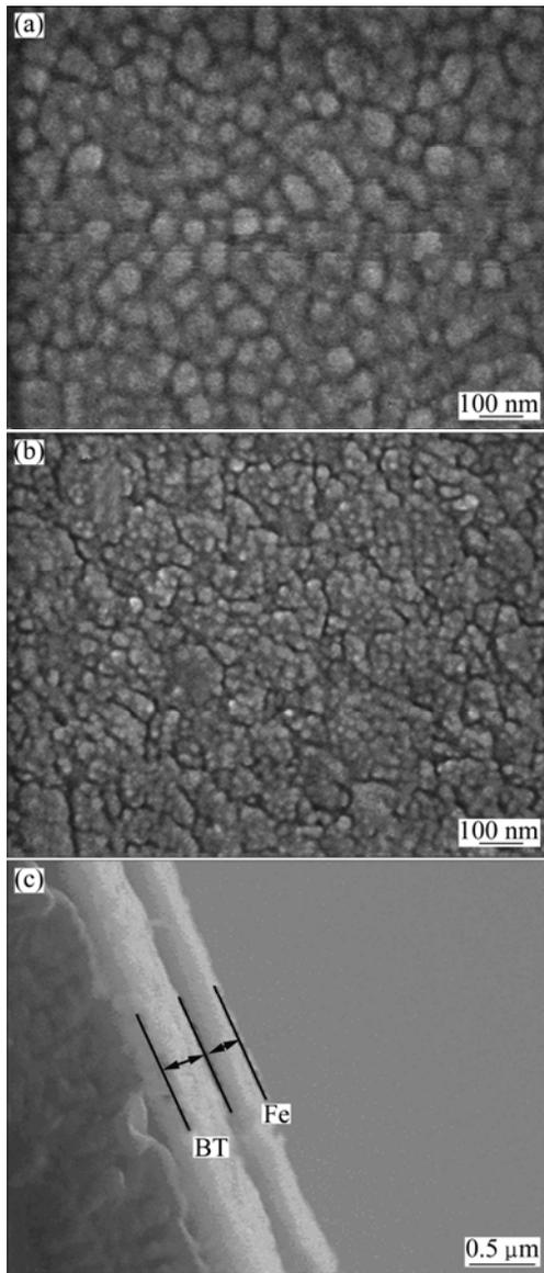
**Fig.2** SEM surface micrographs of BT(001) film (a), Fe(110)/BT(001) film (b), and cross-section image of Fe(110)/BT(001) film (c)
