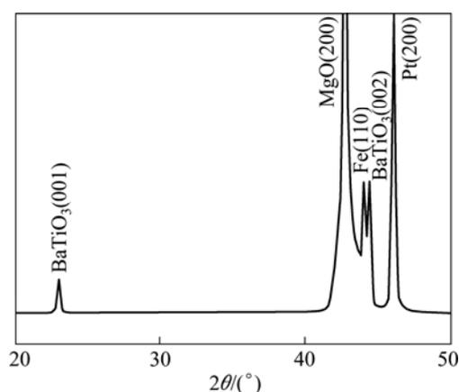
**Fig.1** XRD pattern of bi-layer Fe/BaTiO<sub>3</sub> thin film on Pt(200)/MgO(100) substrate
