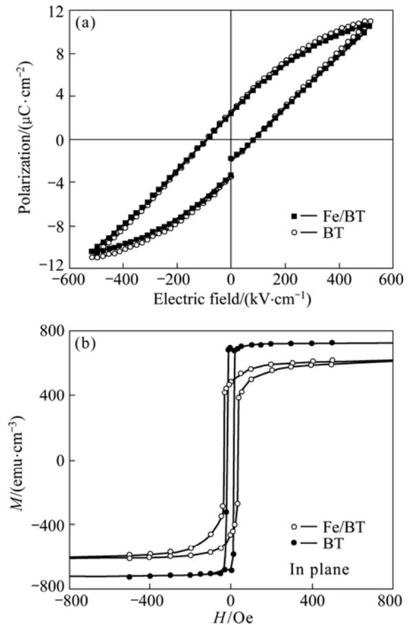
**Fig. 3** Ferroelectric hysteresis loops (a) and in-plane magnetic hysteresis loops (b) of Fe(110)/BT(001) film and pure Fe(110) film
