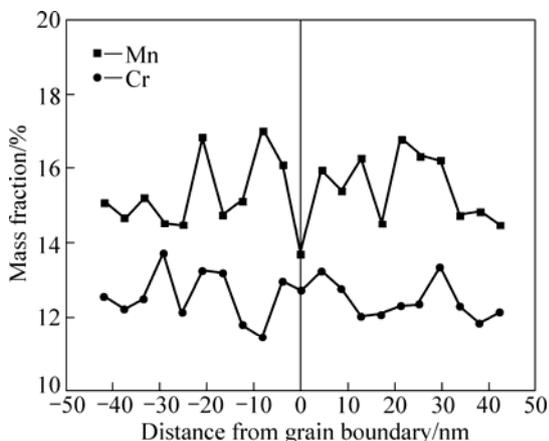
**Fig.4** Comparison of concentration profile near grain boundary after electron-beam irradiation dose up to 5.4 dpa in high Mn-Cr steel aging treated at 573 K for 1000 h
