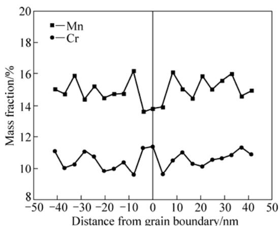
**Fig.3** Comparison of concentration profile near grain boundary after electron-beam irradiation dose up to 5.4 dpa at 573 K in solution treated high Mn-Cr steel
