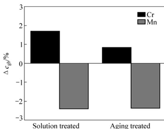
**Fig.5** Comparison of irradiation induced segregation near grain boundary with electron-beam irradiation dose up to 5.4 dpa at 573 K in solution treated and aging treated high Mn-Cr steel
