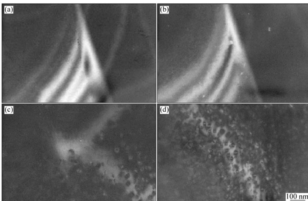
**Fig.2** Microstructure changes of high Mn-Cr steel aging treated after electron-beam irradiation doses up to 0 dpa (a), 1.8 dpa (b), 3.6 dpa (c) and 5.4 dpa (d) at 573 K
