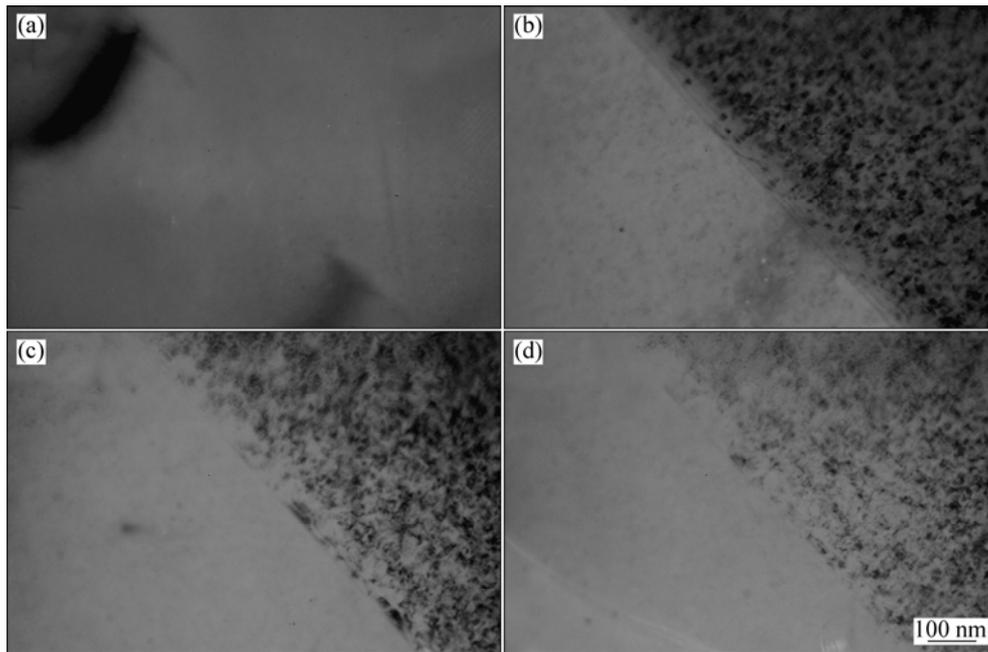
**Fig.1** Microstructure changes of solution treated high Mn-Cr steel after electron-beam irradiation doses up to 0 dpa (a), 1.8 dpa (b), 3.6 dpa (c) and 5.4 dpa (d) at 573 K
