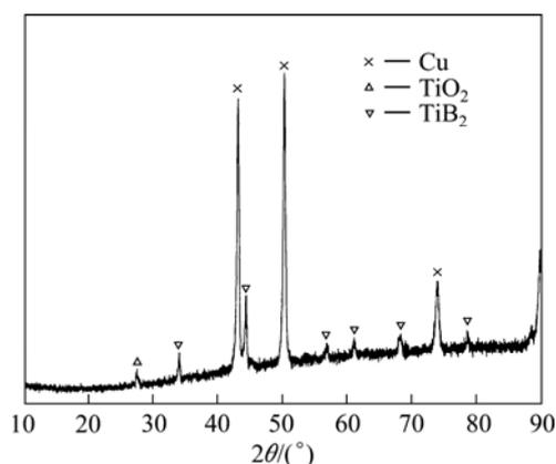
**Fig.5** XRD pattern of  $\text{TiB}_2$  coating
