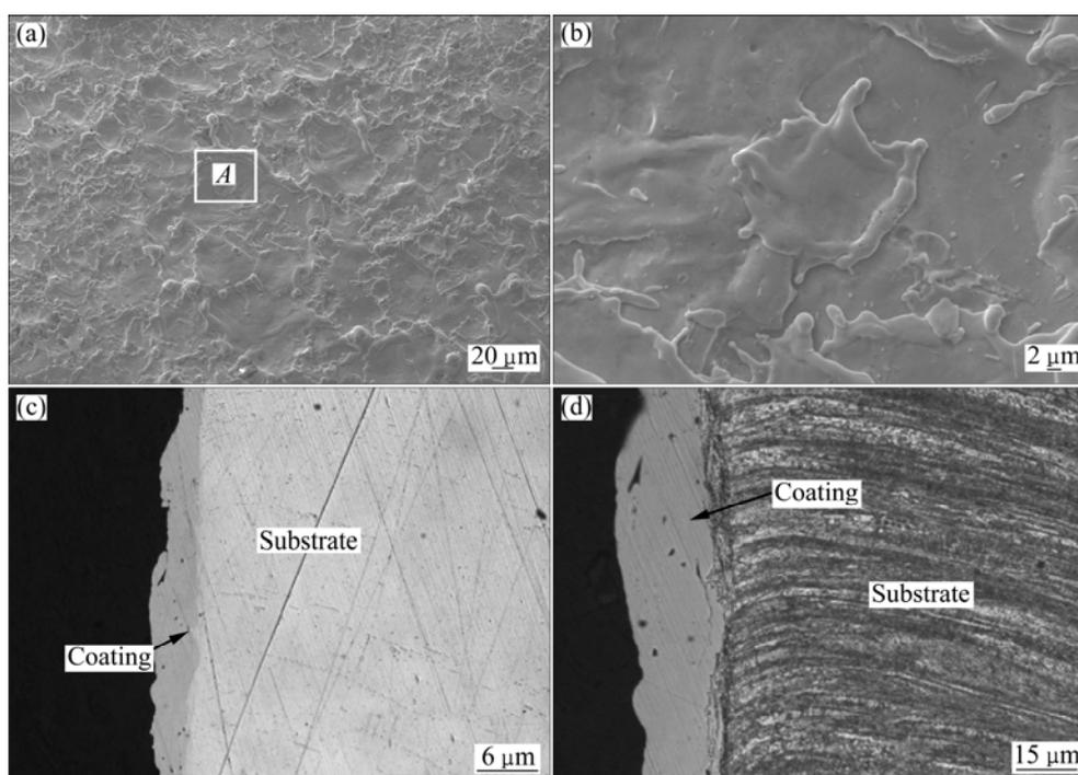
**Fig.1** SEM images of surface of pre-coated nickel (a), enlarged area of A (b), cross section (c) and cross section etched with 5% FeCl<sub>3</sub> solution (d)
