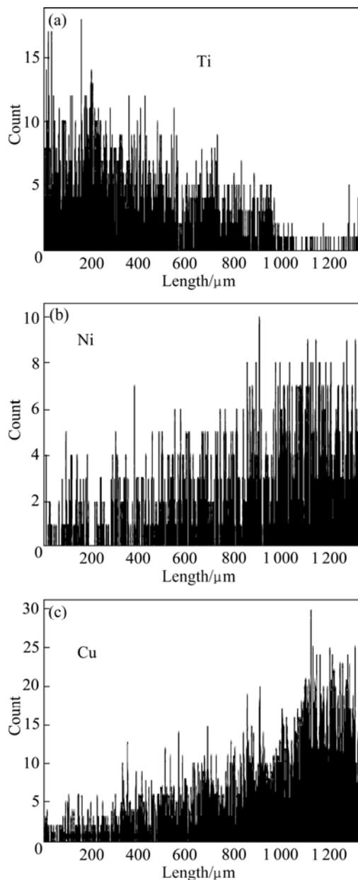
**Fig.4** Linear scanning results for cross-section of  $\text{TiB}_2/\text{Ni}$  coating, for Ti (a), Ni (b), Cu (d)
