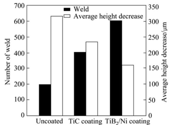
**Fig.6** Spot-welding lives for electrodes with different coatings and their average height decreases
