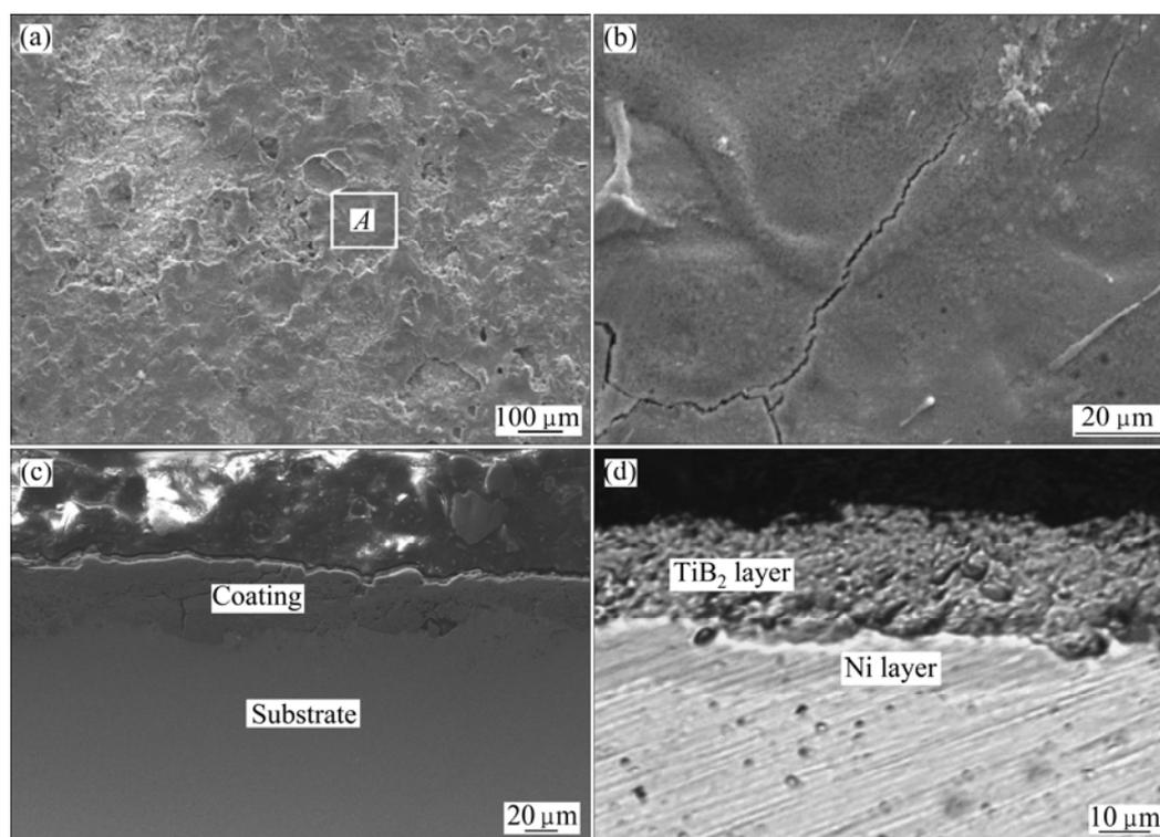
**Fig.3** SEM images of  $\text{TiB}_2/\text{Ni}$  coating surface (a), enlarged area of A (b), cross section (c) and optical microscopy of cross section (d)
