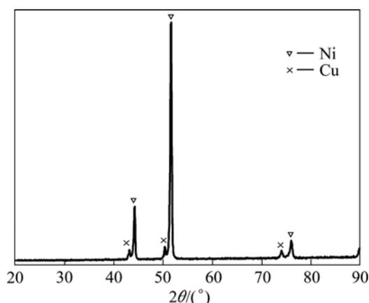
**Fig.2** XRD pattern of top surface of precoated nickel
