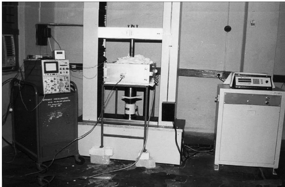
Fig.2 Servo controlled universal testing machine used for hot compression test
