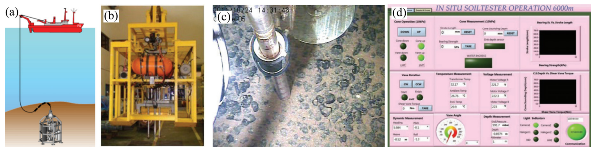
图 9 深海底质原位测试系统 [39] Fig. 9 In-situ testing system of deep-sea sediment [39] : (a) Model; (b) Tester; (c) Test procedure; (d) Operation interface
