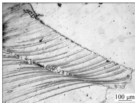
Fig.7 Microstructure obtained on Ti40 alloy specimens deformed in instability regime showing manifestations in form of shear bands on deformation at 950 °C and 10 s -1
