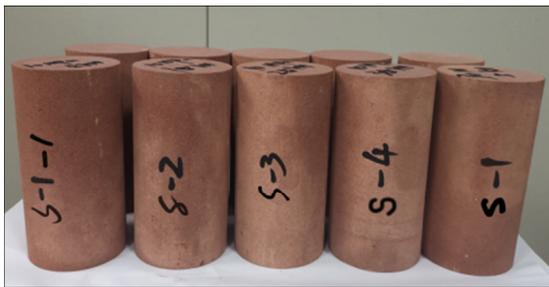
**Fig. 2** Red sandstone cylinder specimens in permeability test
