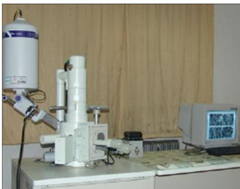
**Fig. 7** JSM-6360LV scanning electron microscope
