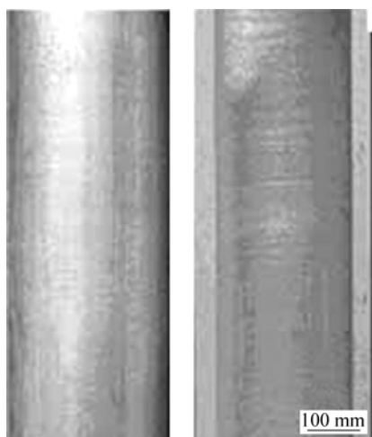
Fig.10 \phi 350 mm \times 30 mm 6061 alloy hollow billets cast by HBEC
