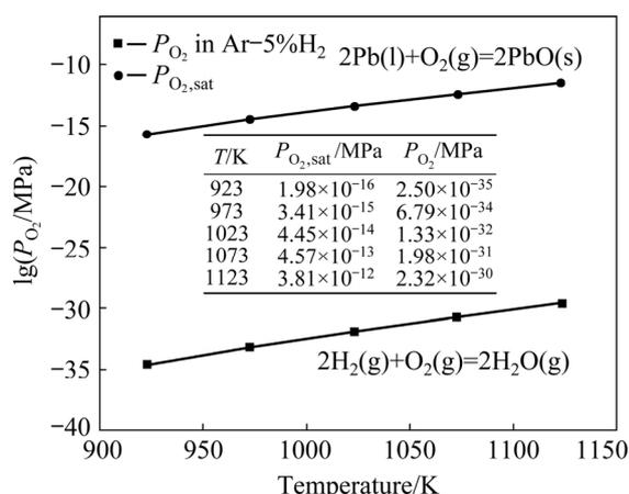
**Fig. 9** Oxygen partial pressure in Ar-5% $H_2$  atmosphere and equilibrium oxygen partial pressure of Pb/PbO system
