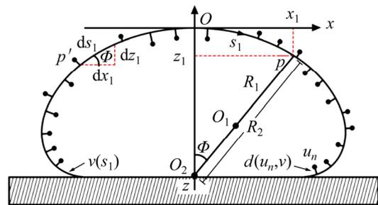
**Fig. 1** Theoretical model of surface tension measurement with sessile drop method
