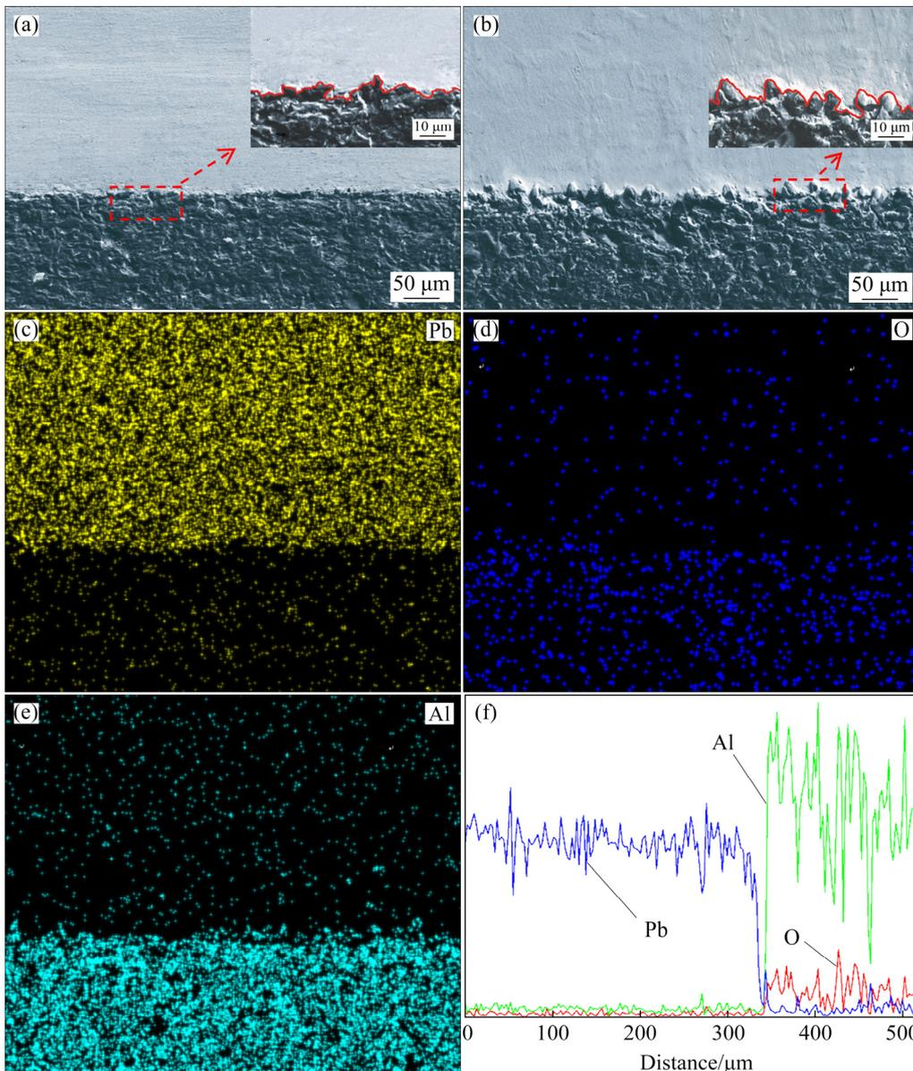
**Fig. 5** SEM images (a, b) of interface between lead and alumina substrate, corresponding element distribution maps (c–e) in (a), and linear scanning analysis (f): (a)  $R_a=0.092\ \mu\text{m}$ ; (b)  $R_a=2.23\ \mu\text{m}$
