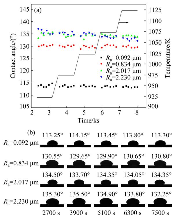
**Fig. 3** Changes for contact angle of lead drop on alumina substrate with different roughnesses at various temperatures (a), and wetting morphologies at 2700, 3900, 5100, 6300 and 7500 s with different roughnesses (b)
