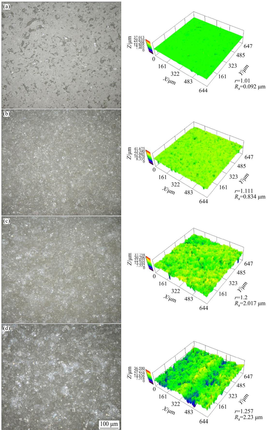
**Fig. 2** CLSM analysis for different alumina substrates surface: (a) 1#; (b) 2#; (c) 3#; (d) 4#
