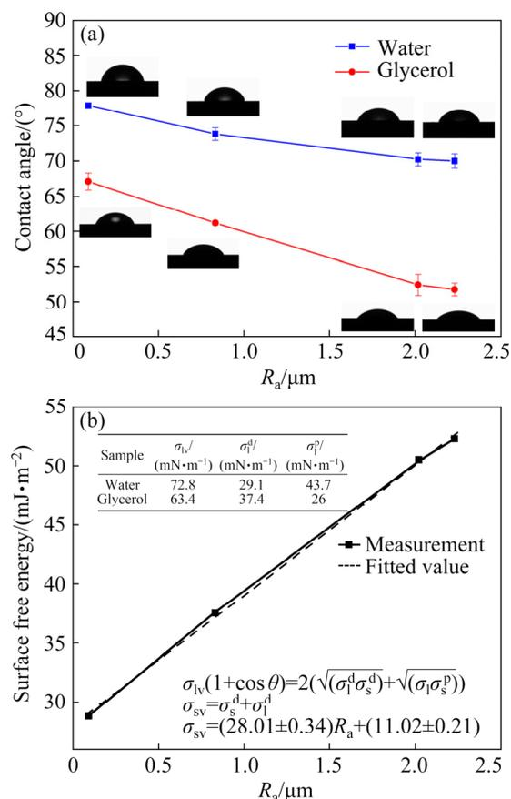
**Fig. 7** Contact angle of deionized water and glycerol on alumina substrate of different roughnesses with maximum error of  $\pm 2\%$  (a), and relationship between surface free energy and  $R_a$  of alumina substrate (b)
