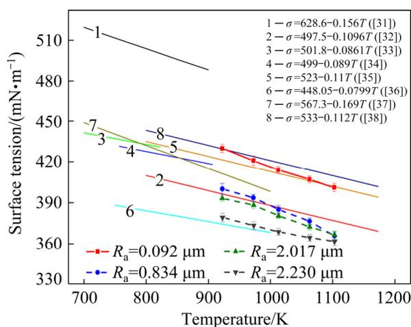
**Fig. 8** Temperature dependence of surface tension of lead and roughness dependence of surface tension of lead from experimental data
