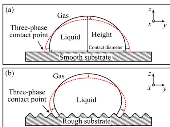
**Fig. 6** Wetting of drop on smooth substrate (a) and on rough substrate (b)
