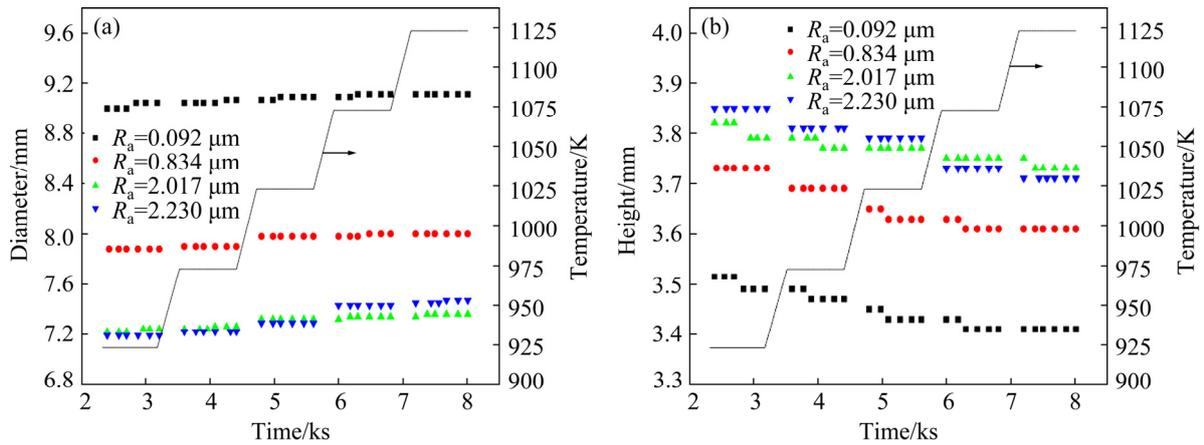
**Fig. 4** Changes for contact diameter (a) and droplet height (b) of lead drop on alumina substrate with different roughnesses at various temperatures
