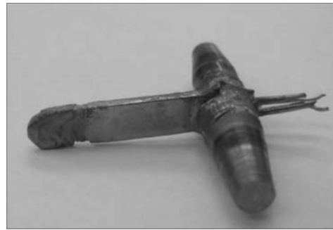
Fig.5 Example of demonstrator in initial stage of mini thixoforming development with incomplete filling of die cavity
