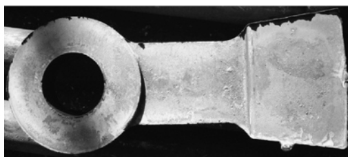
Fig.2 Hammer produced by semisolid rheo-squeeze casting process
