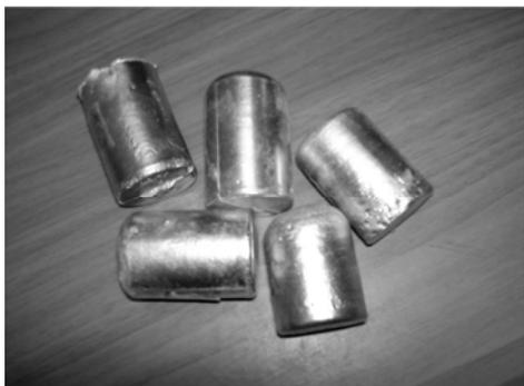
Fig.1 Billets of SiC<sub>p</sub>/A356 composites
