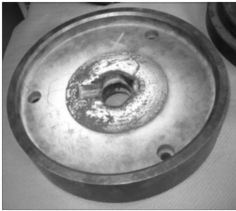
Fig.7 Lower die used for thixoforging experiments with cavity for shapes forging
