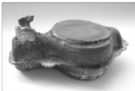
Fig. 11 Part obtained from 100Cr6 steel alloy
