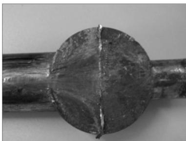
Fig.12 Streamline of workpiece
