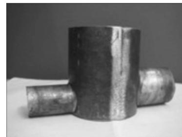
Fig.14 Workpiece formed by semi-solid thixoforging
