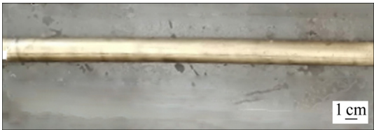
图 2 铝白铜铸坯宏观形貌 Fig. 2 Macrophotology of casting bar of aluminium white copper
