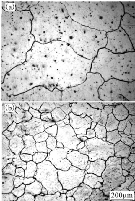
**Fig.6** Solid solution microstructure of AM60 billet from: (a) Metal mold cast; (b) CRP
