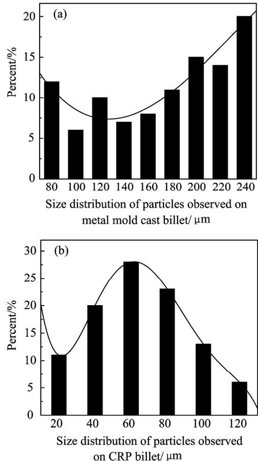
**Fig.7** Size distribution of particles observed on AM60 billet from: (a) Metal mold cast; (b) CRP
