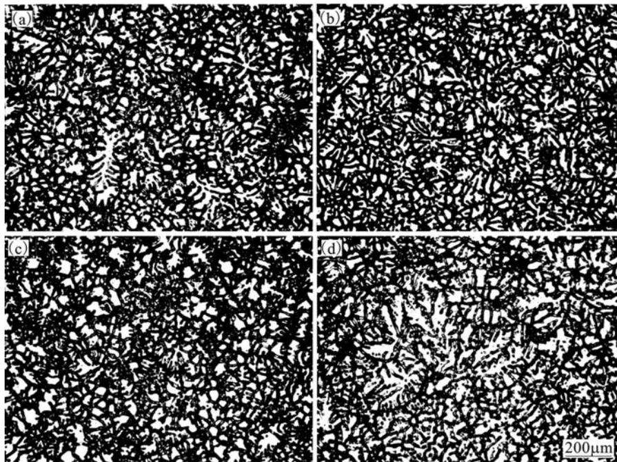
**Fig.4** As-cast microstructures of AM60 billet with CRP at different slope angles of reactor: (a) 15°; (b) 30°; (c) 45°; (d) 60°
