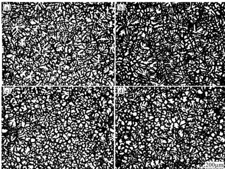
**Fig.3** As-cast microstructures of AM60 billets with CRP at different pouring temperatures: (a) 700 °C; (b) 680 °C; (c) 660 °C; (d) 640 °C
