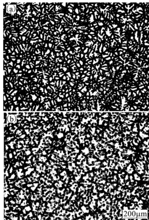
**Fig.5** As-cast microstructures of AM60 billets by using CRP with different lengths of reactor: (a) 500 mm; (b) 850 mm
