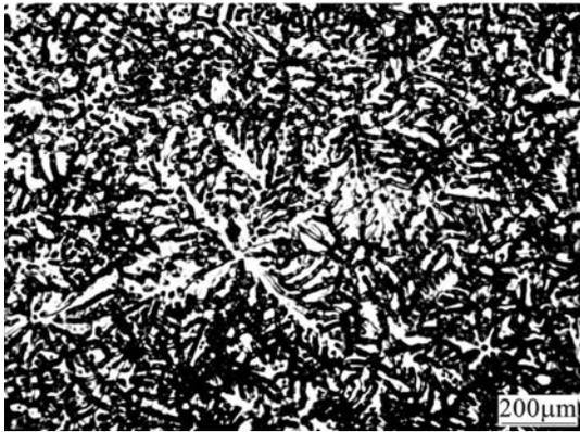
**Fig.2** Typical dendritic microstructure of AM60 alloy during conventional solidification
