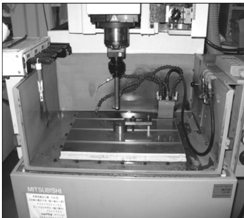
**Fig.10** Engraving electrical discharge machine
