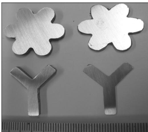
**Fig.6** Sliced samples of shape intended design material of extruded products
