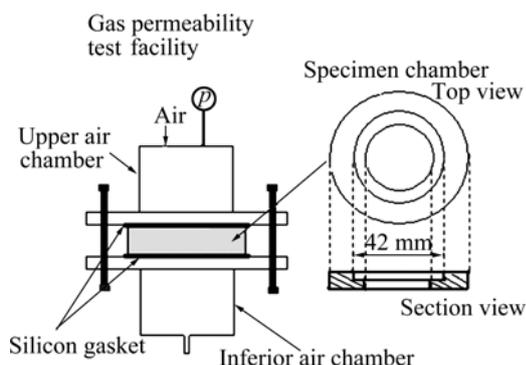
Fig.3 Scheme of gas permeability measurement
