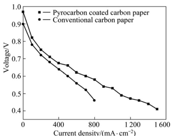
Fig.8 Polarization curves of carbon fiber paper samples
