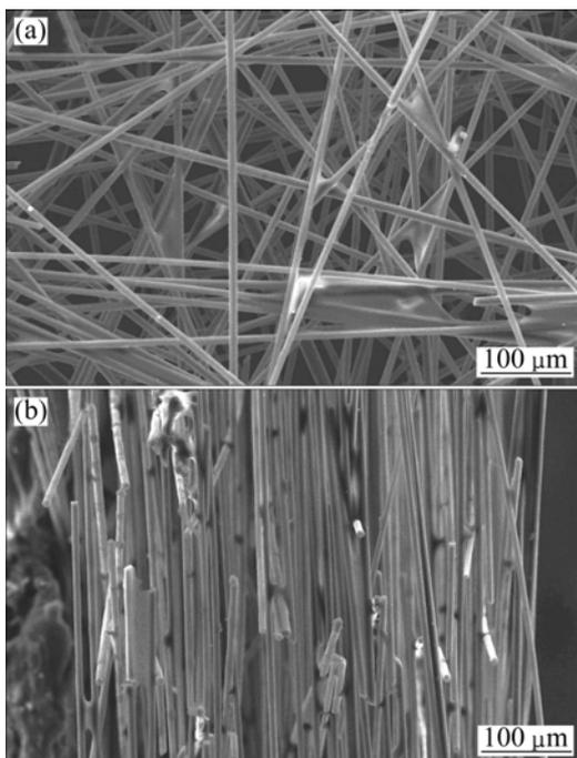
**Fig.1** SEM micrographs of surface (a) and cross-section (b) of carbon fiber felt
