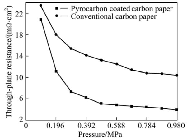
**Fig.6** Variations of through-plane resistances of carbon fiber paper with pressure
