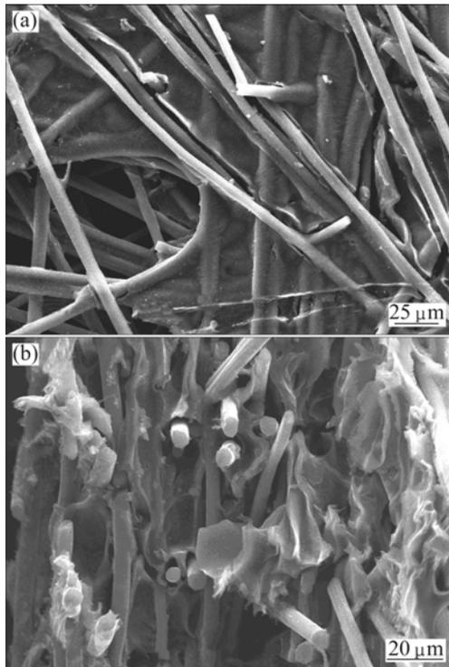
**Fig.5** SEM micrographs of surface (a) and cross-section (b) of conventional carbon paper
