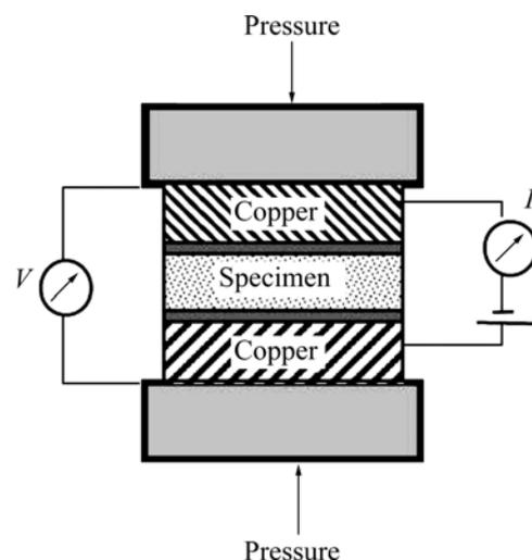
**Fig.2** Scheme of experimental setup used in through-plane resistances measurement
