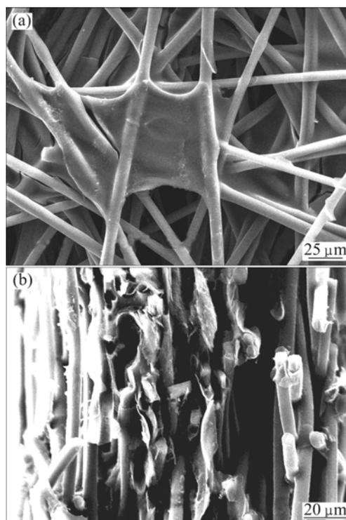
Fig.4 SEM micrographs of surface (a) and cross-section (b) of pyrocarbon coated carbon paper
