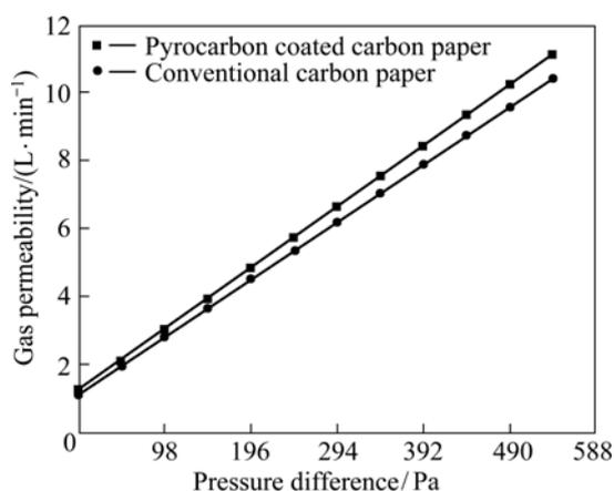
Fig.7 Variations in gas permeability of carbon fiber paper with pressure difference
